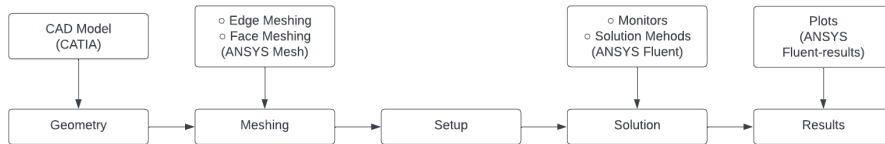
Figure 3.3: CFD Process Flowchart
