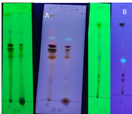
Figure 4.17: TLC plate of (A) hexane and methanol extract in 35% acetone in hexane and (B) hexane extract in 20% ethylacetate in hexane
