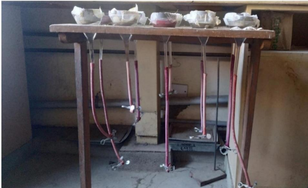
Photograph 2: Baermann funnel set up for extraction of nematodes.
