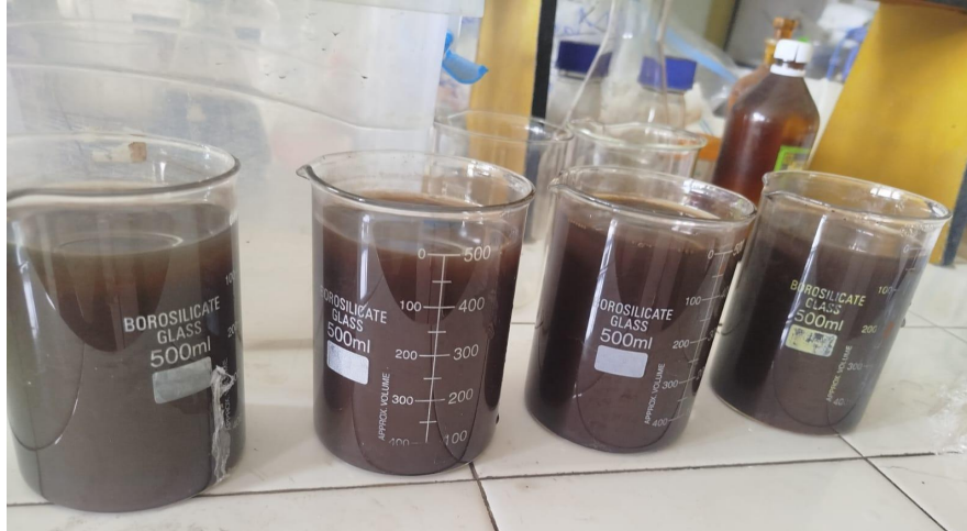
Figure 3. 3: CuO-Al_2O_3 -water after sonication
