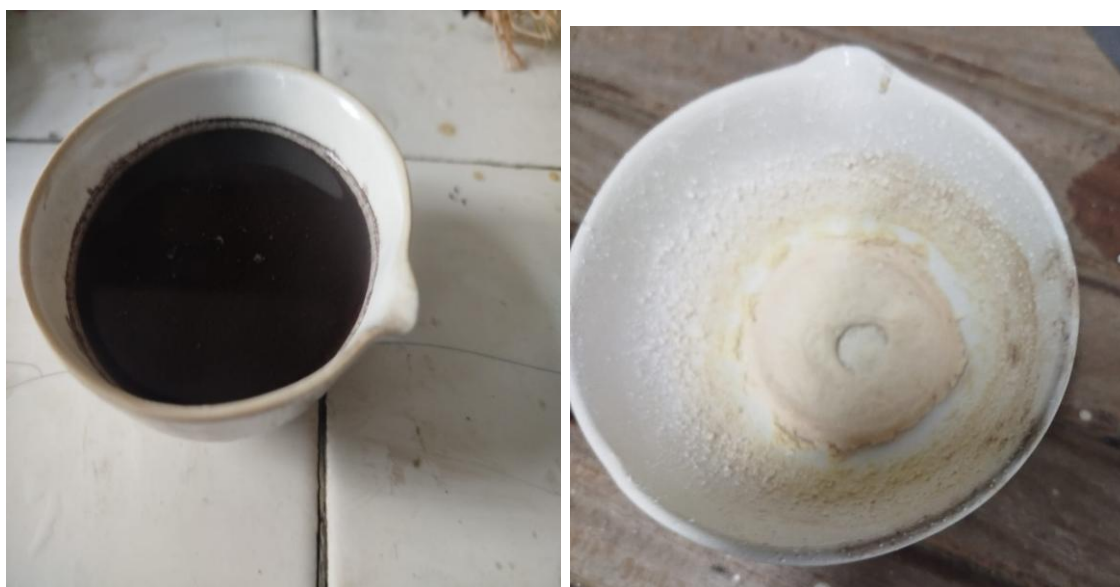
Figure A2. 2: Gel-stage of CuO (left) and Al 2 O 3 (right)
