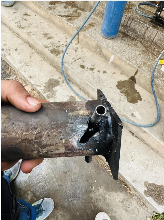
Figure 4.8: Chamber and oxygen injector failure
