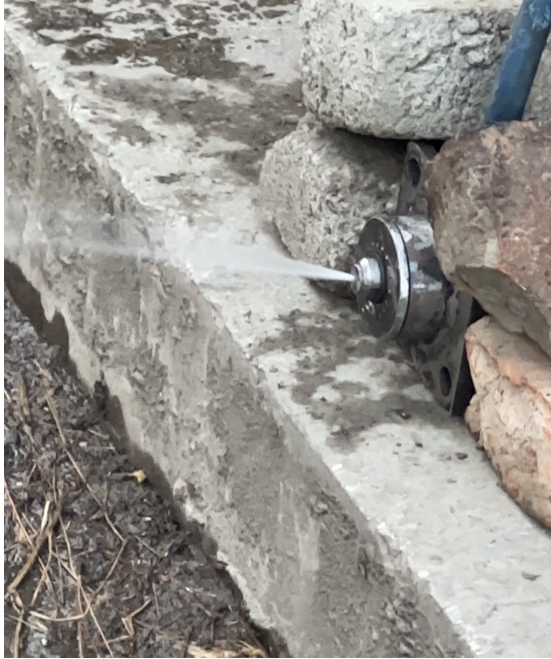
Figure 4.10: Injector test with water
