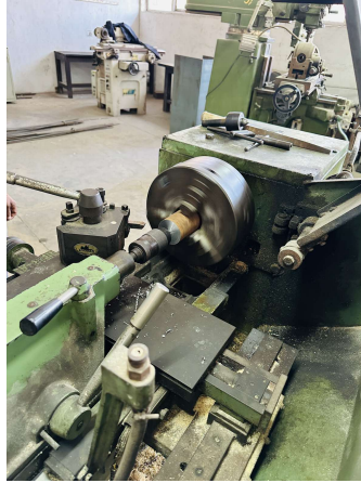
Figure 3.9: Injector Drilling Process
