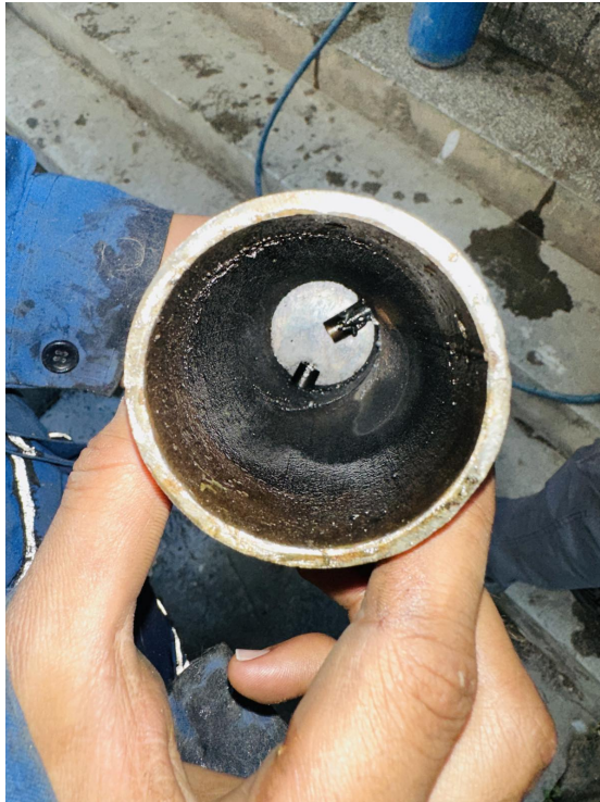
Figure 4.7: Charring of the combustion chamber after the test
