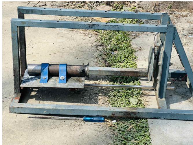
Figure 3.7: Thrust stand (Courtesy of SRB ,IOE Pulchowk)
