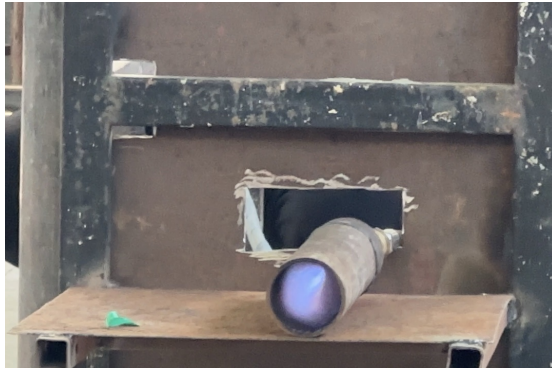
Figure 4.2: Blue flame (LPG + GOX)
