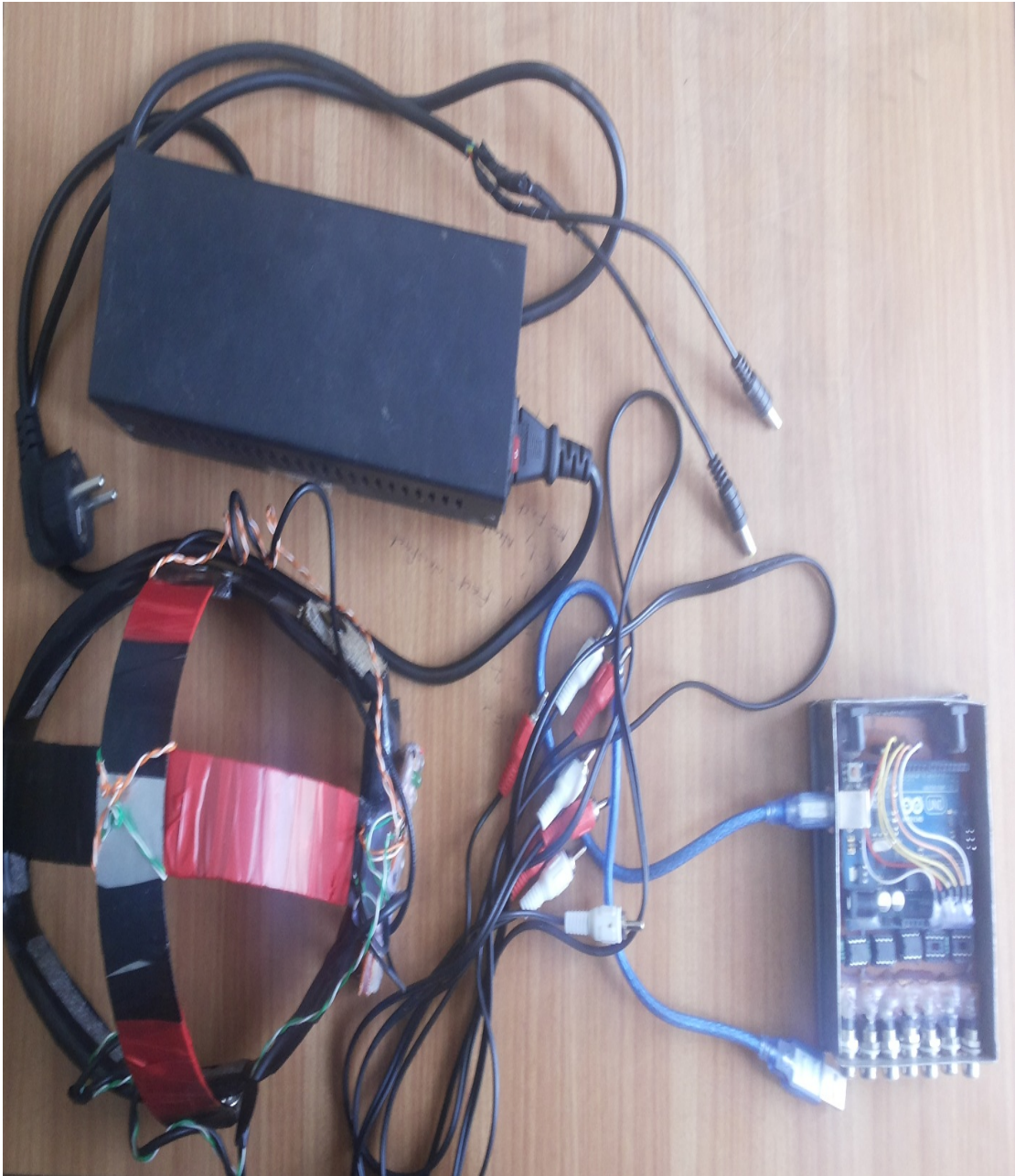
Figure A.1: Different components of a 3-channel EEG Device for recording brainwaves which includes a power supply, an EEG headset and an amplifier.
