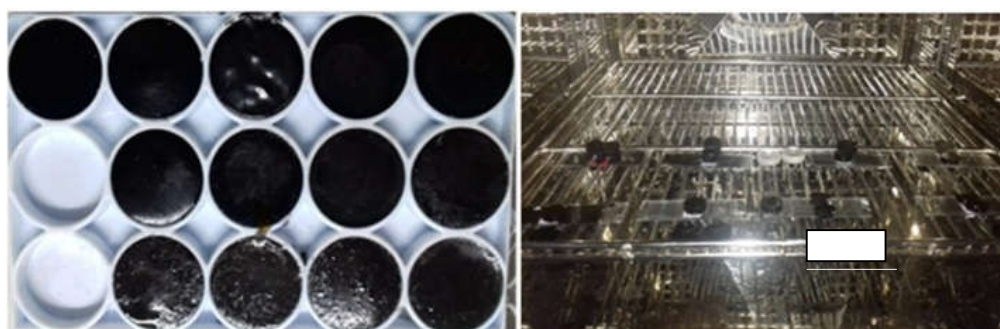
Figure 35: Epoxy/nanocarbon nanocomposites procured at plastic mould for 24 hrs at room temperature (25 °C)
