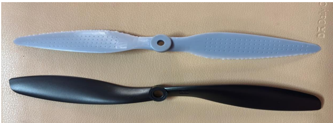
Figure 3.14: Commercially available propeller on the left and resin printed one on the right
