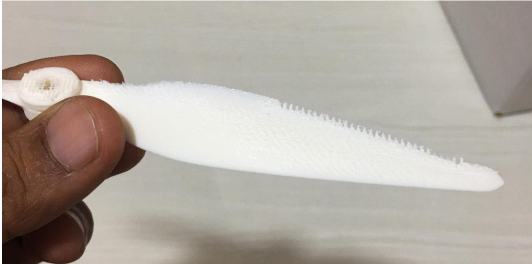
Figure 3.13: PLA prop with severe imperfections
