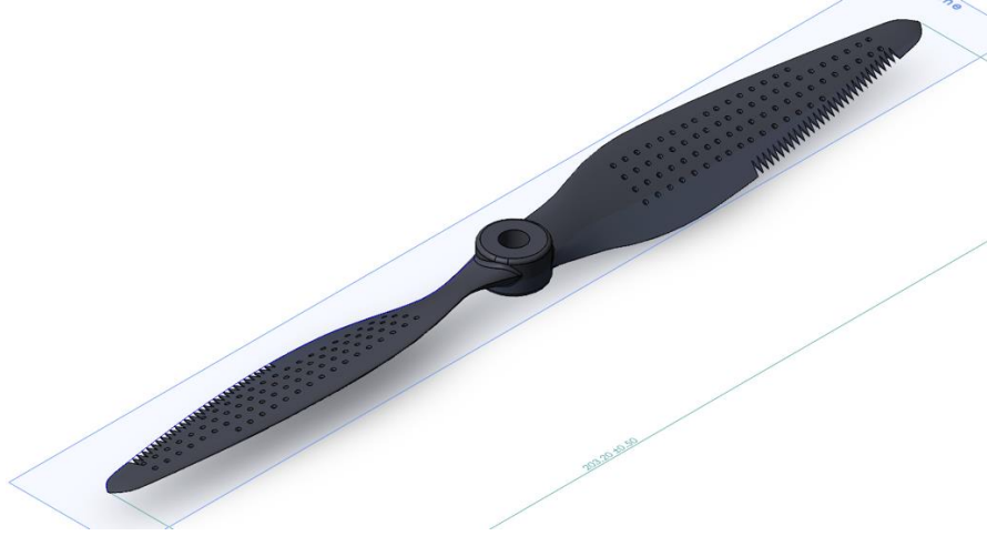
Figure 3.7: Serrated trailing edge and circular dimpled propeller model
