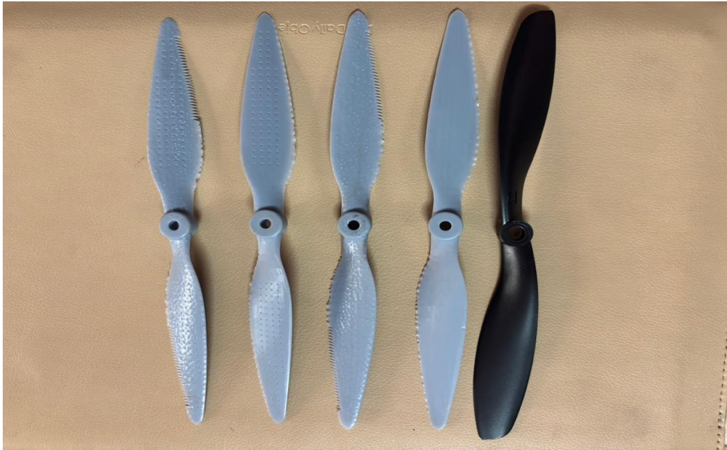
Figure 3.15: Resin Printed Propellers and commercial propeller
