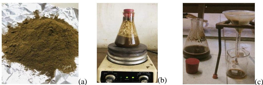
Figure 10: Preparation of Lawsonia inermis Extract for Carbon Dot Synthesis. a) Lawsonia inermis leaves powder, b) Extraction process in progress, c) Filtration of the extract
