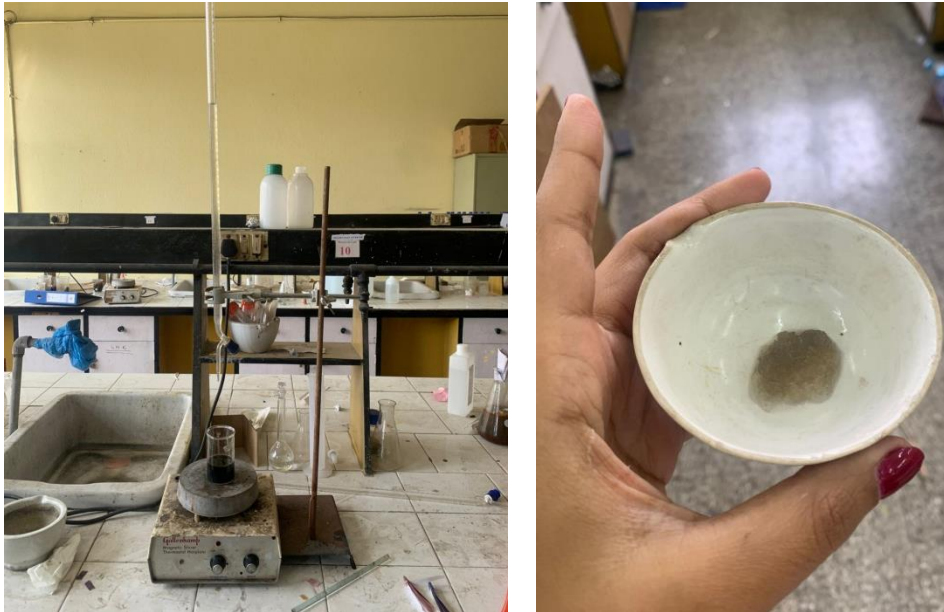
Figure 3.5: Adding HCL drop wise to get silica gel
