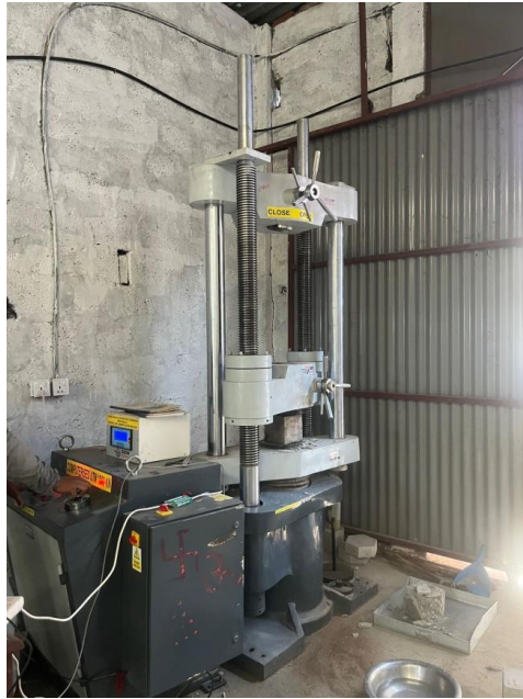
Figure 3.19: Compressive strength Apparatus
