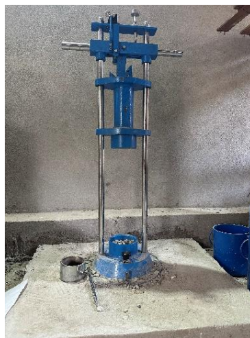
Figure 3.13: Impact test Apparatus
