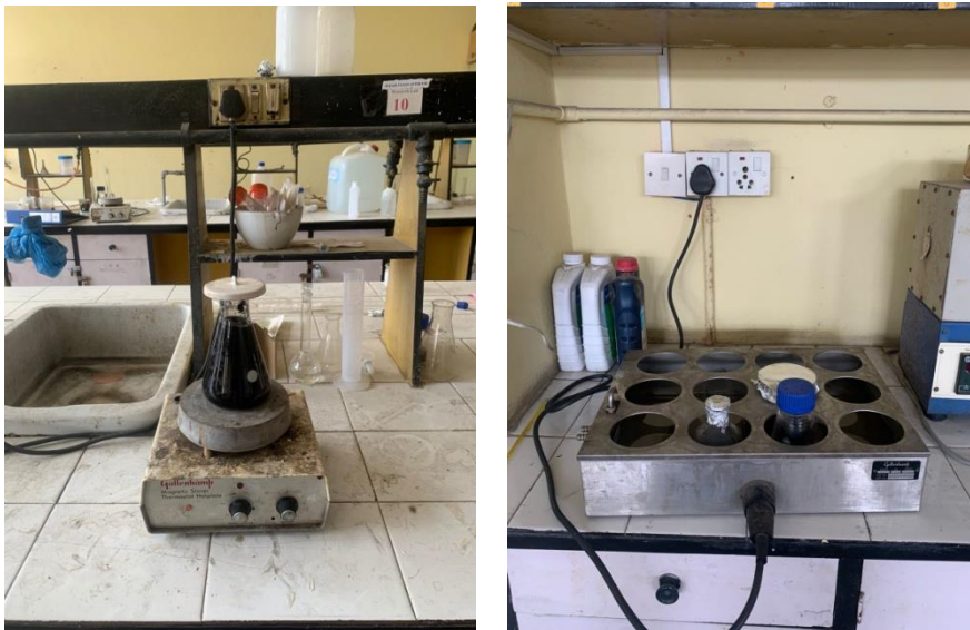
Figure 3.4: Heating and Mixing of Rice husk ash with KOH
