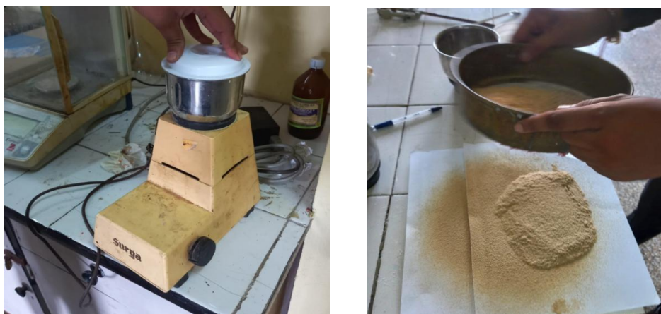
Figure 3.2: Grinding of the Sample into its appropriate size
