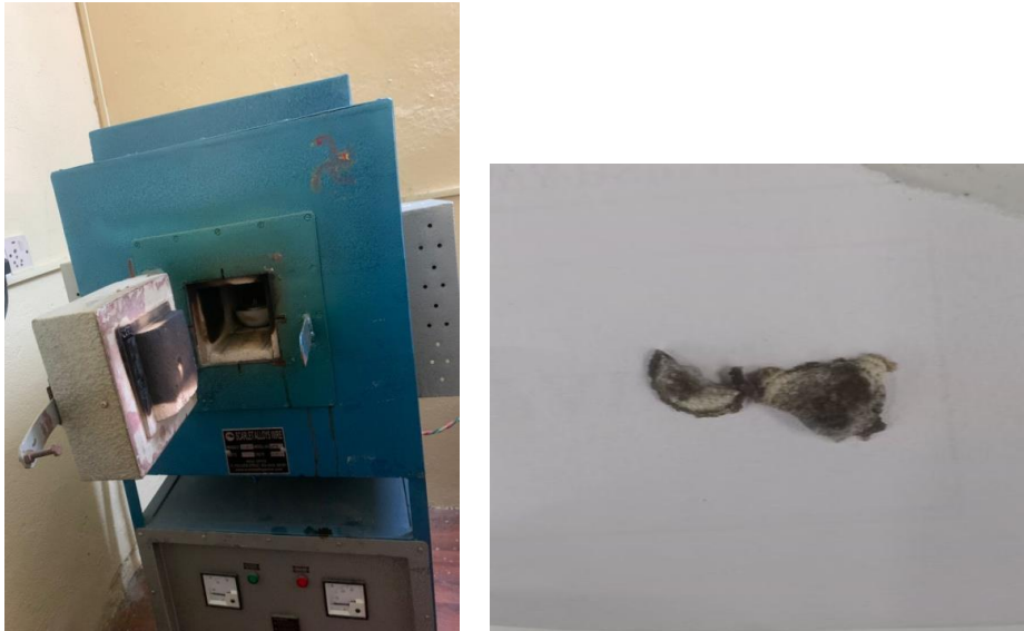
Figure 3.6: Drying and formation of silica
