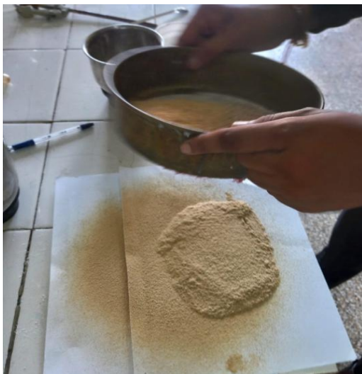
Figure: preparation of Rice husk ash
