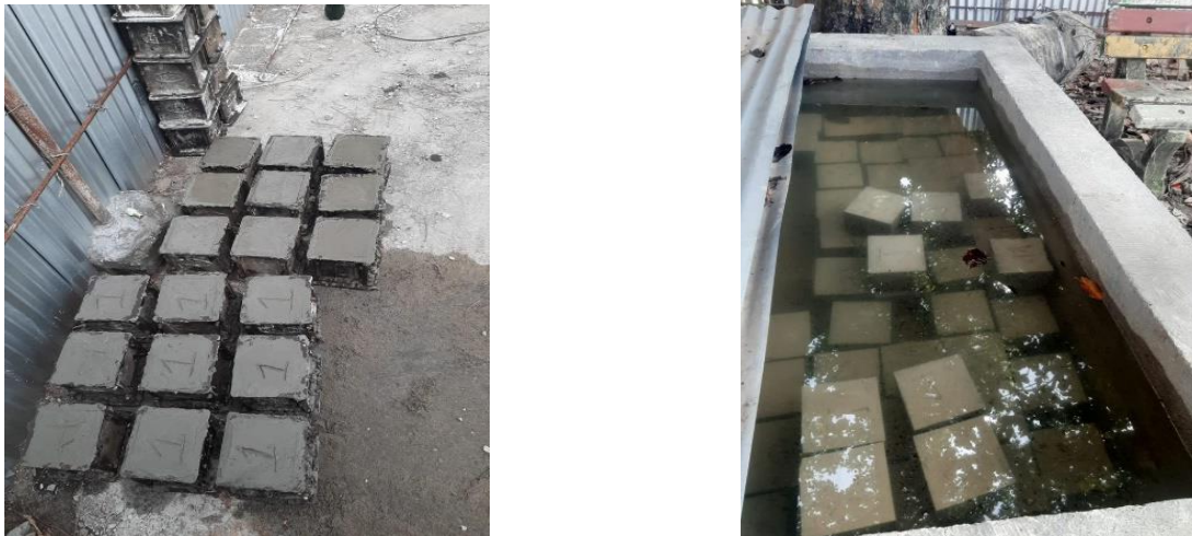
Figure 3.18: Placing and Curing of Cubes
