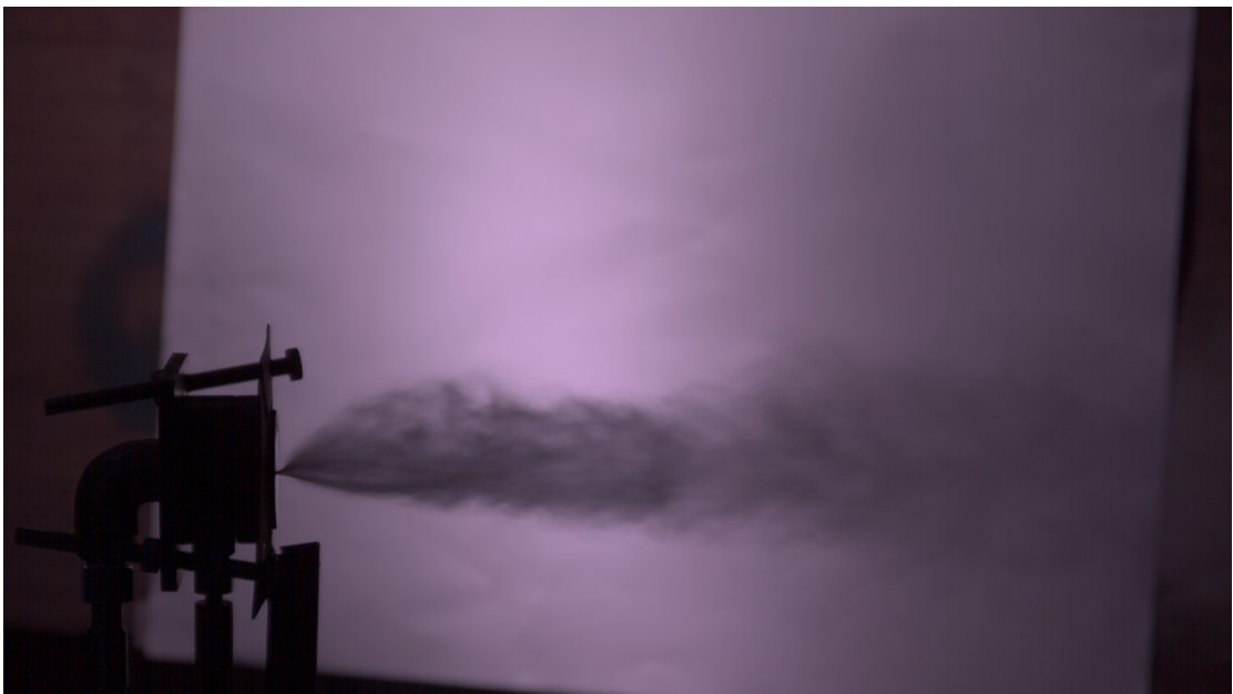
Figure 4.28: Cold flow testing of 1 on 1 impingement injector at 150 psi
