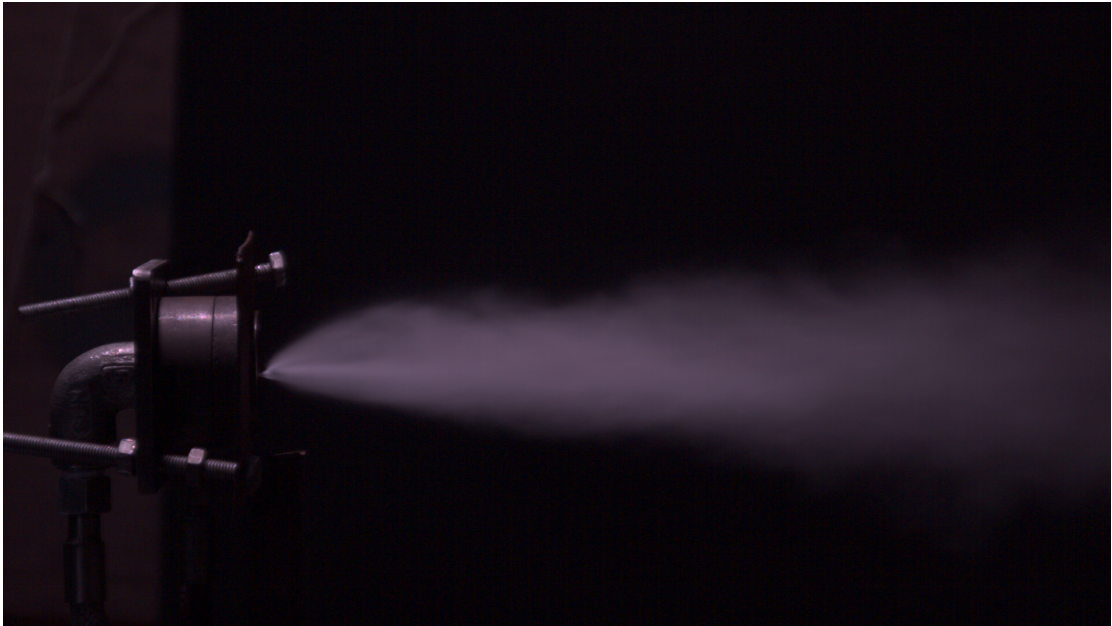
Figure 4.27: Cold flow testing of 1 on 1 impingement injector at 50 psi
