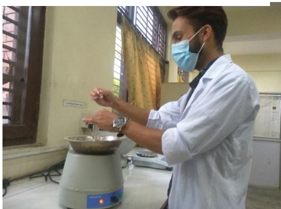
Figure 3: Performing sample digestion for determination of phosphorus and trace elements
