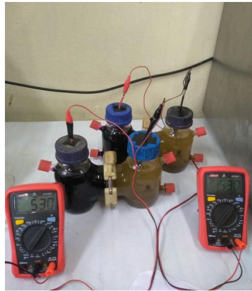
Figure 2: Dual chambered MFC operation at Biofuel lab of CDBT
