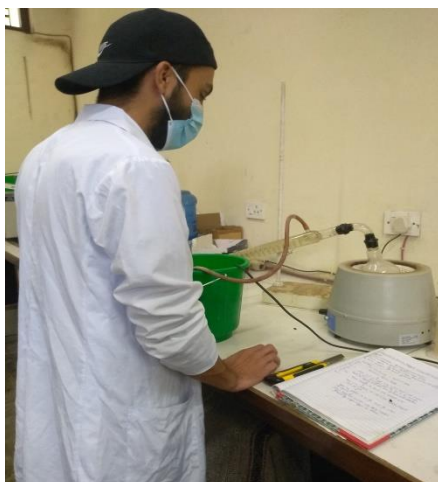
Figure 5: Carrying out distillation during ammoniacal- nitrogen determination
