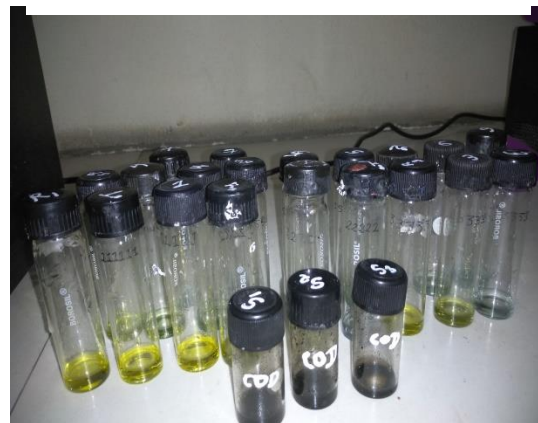
Figure 4: Colour observed after digestion during COD determination
