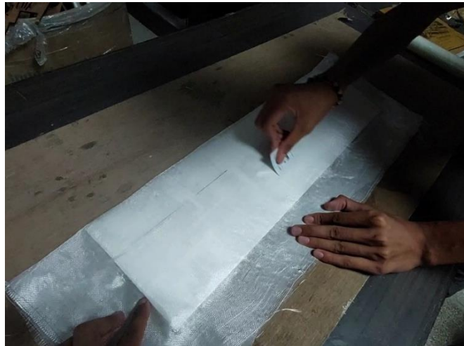
Wet layup of fiberglass with resin using a spreader
