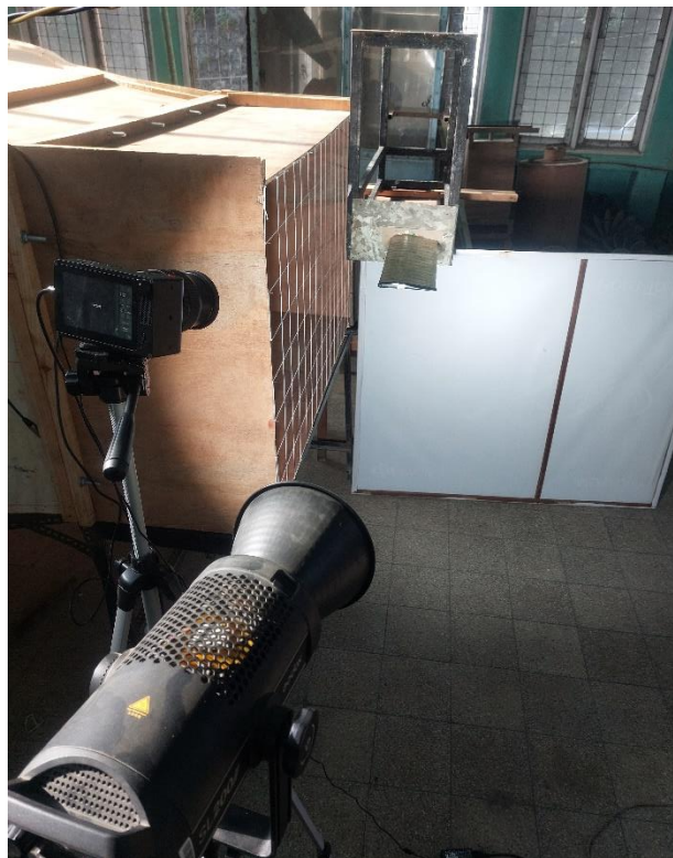
Figure 3.12: Experimental Setup for Wind Tunnel Testing of the Wing
