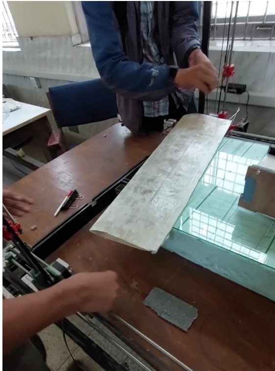
Removal of the foam core from the skin using hotwire
