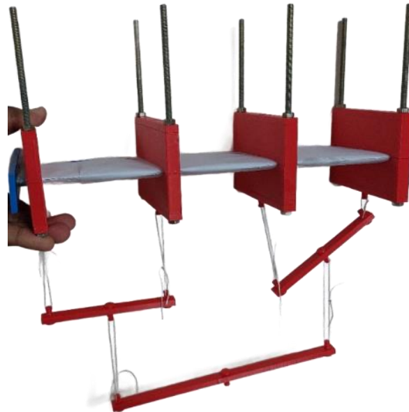
Figure 3.9: 1:2 scale 3D-Printed model of the whiffletree test rig
