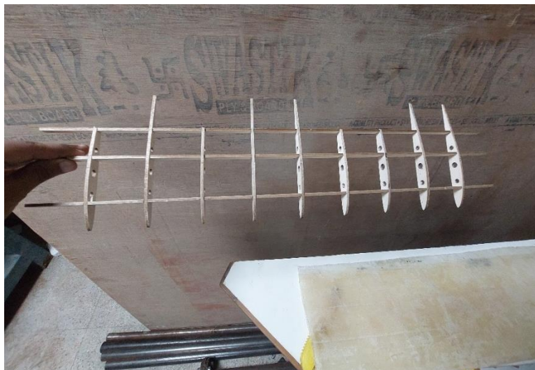
3.175mm thick balsa frame structures failing during assembly due to design flaws.
