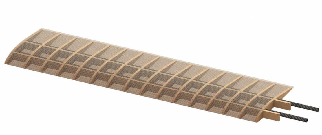
Figure 4.2: CAD model of the designed wing with 5mm thick balsa structures (3D rendered view)
