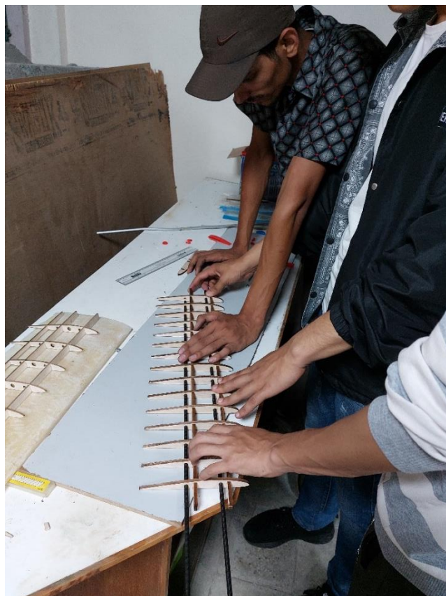
Assembling carbon fiber rod with balsa frame structure for improvised design
