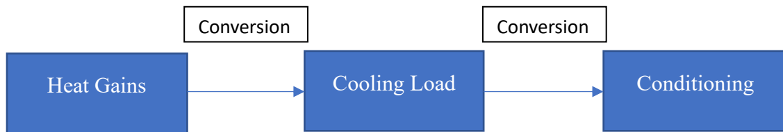
Figure 2.2: Heat balance process flow diagram
