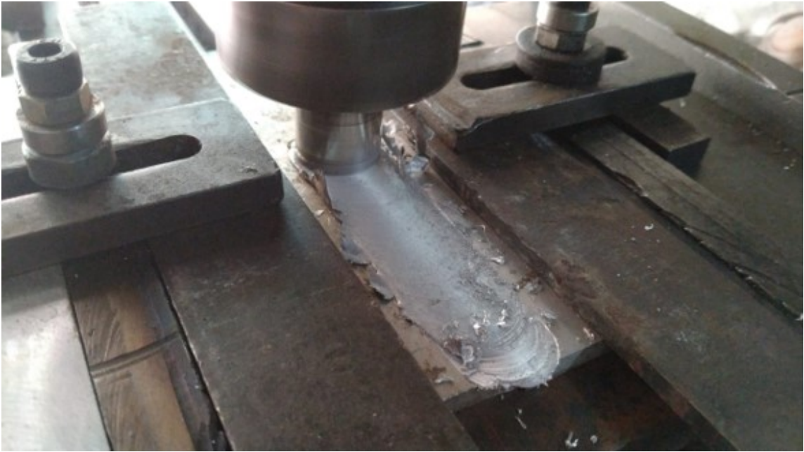
Sample Obtained after Cutting the Welded Joint
