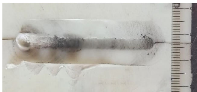
Figure 4-1: Spindle Speed at 180 rpm (Front View)
