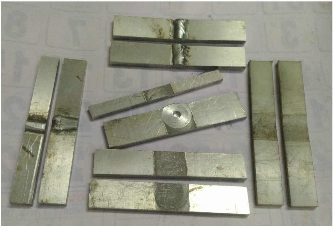
Sample Obtained after Cutting the Welded Joint
