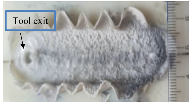
Figure 4-3: Spindle Speed at 250 rpm (Front View)
