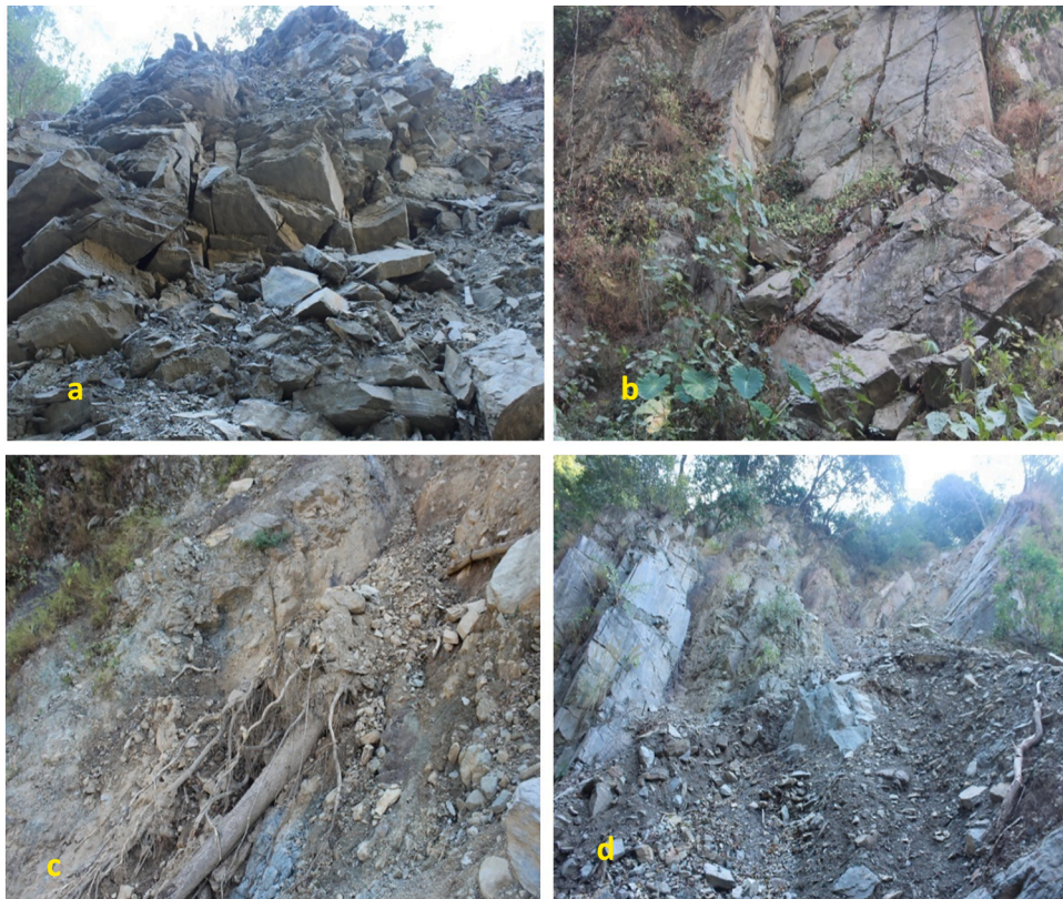
Fig. 11. a) Fragile and broken rocks of Middle Siwalik (hanging wall of Babai thrust) b) Plain failure on the highly jointed rocks of thrust zone c) Uprooted tree on the landslide of hanging wall d) Landslide occurred on the alternate bed of sandstone and mudstone.
