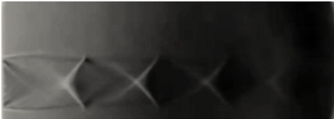
(b) Z-type Schlieren visualization [3]
