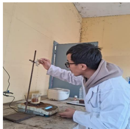
Weighing the suspended sample
