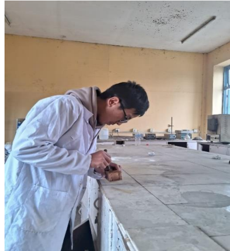
Casting geopolymer sample
