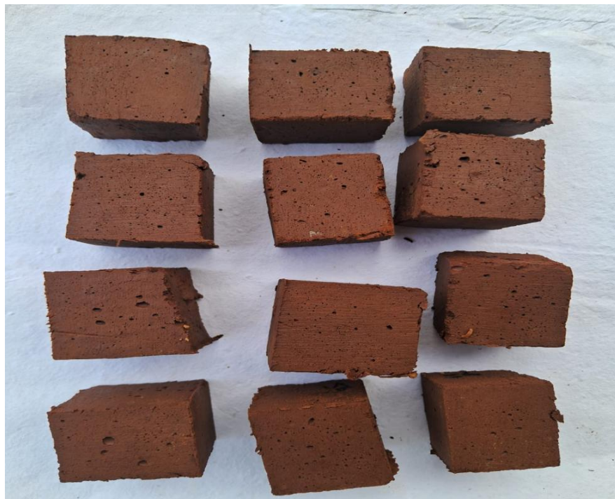
Figure 14: Preparation of geopolymer cubes (RC-2)
