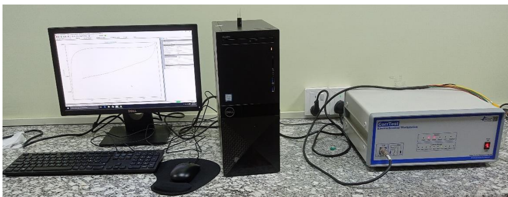
Figure 5: Digital image of Potentiostat Workstation at the Department of Applied Science and Chemical Engineering, Pulchok, IOE, TU
