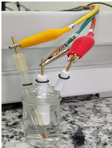
Figure 6: Digital image of the arrangement of three electrodes in potentiostat for cyclic voltammetry measurement.
