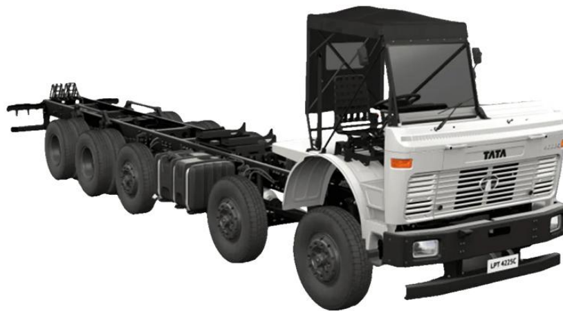
Figure 4.4: LPT 4225.T BSVI COWL 10*2 tridem rear axle heavy vehicle
