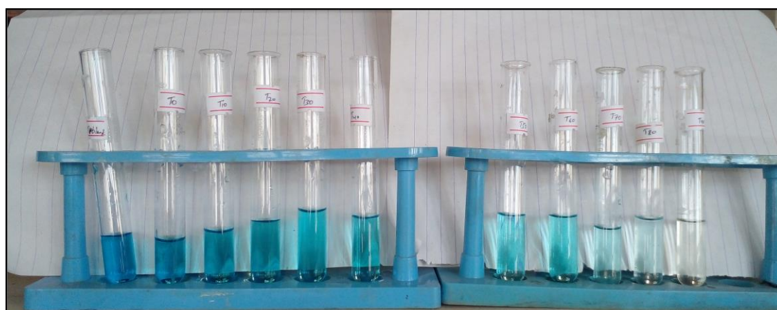
Figure 4.7: Photographic image of the MB dye degradation photocatalytically at different intervals of time by plant-mediated synthesized IONPs.
