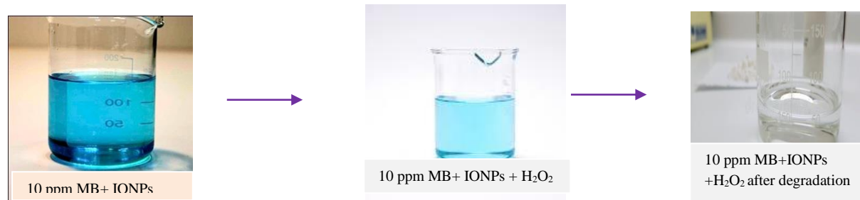
Figure 4.6: Photocatalytic degradation of 10 ppm Methylene blue by plant-mediated synthesized IONPs.
