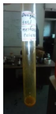
dragendroff test of methanol extract
