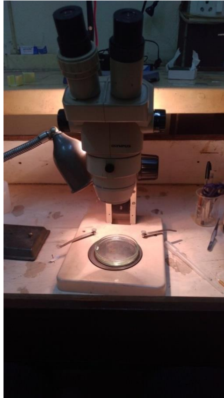
Photograph 3: Stereoscopic Microscope used for nematode extraction from water collected from Baermann set up.
