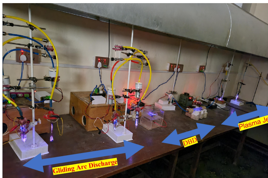
Figure 22: CAPP reactors at plasma research lab at Central Department of Physics, Tribhuvan University, Kirtipur, Nepal
