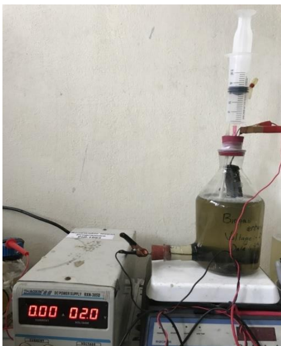
Figure 4.1 : Aspirator bottle used for the anaerobic digestion which served feasible not only for sampling and maintenance of anaerobic state but also for conduction of microbial electrochemical cell.
