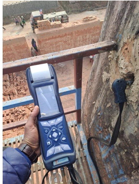
Flue gas analysis
