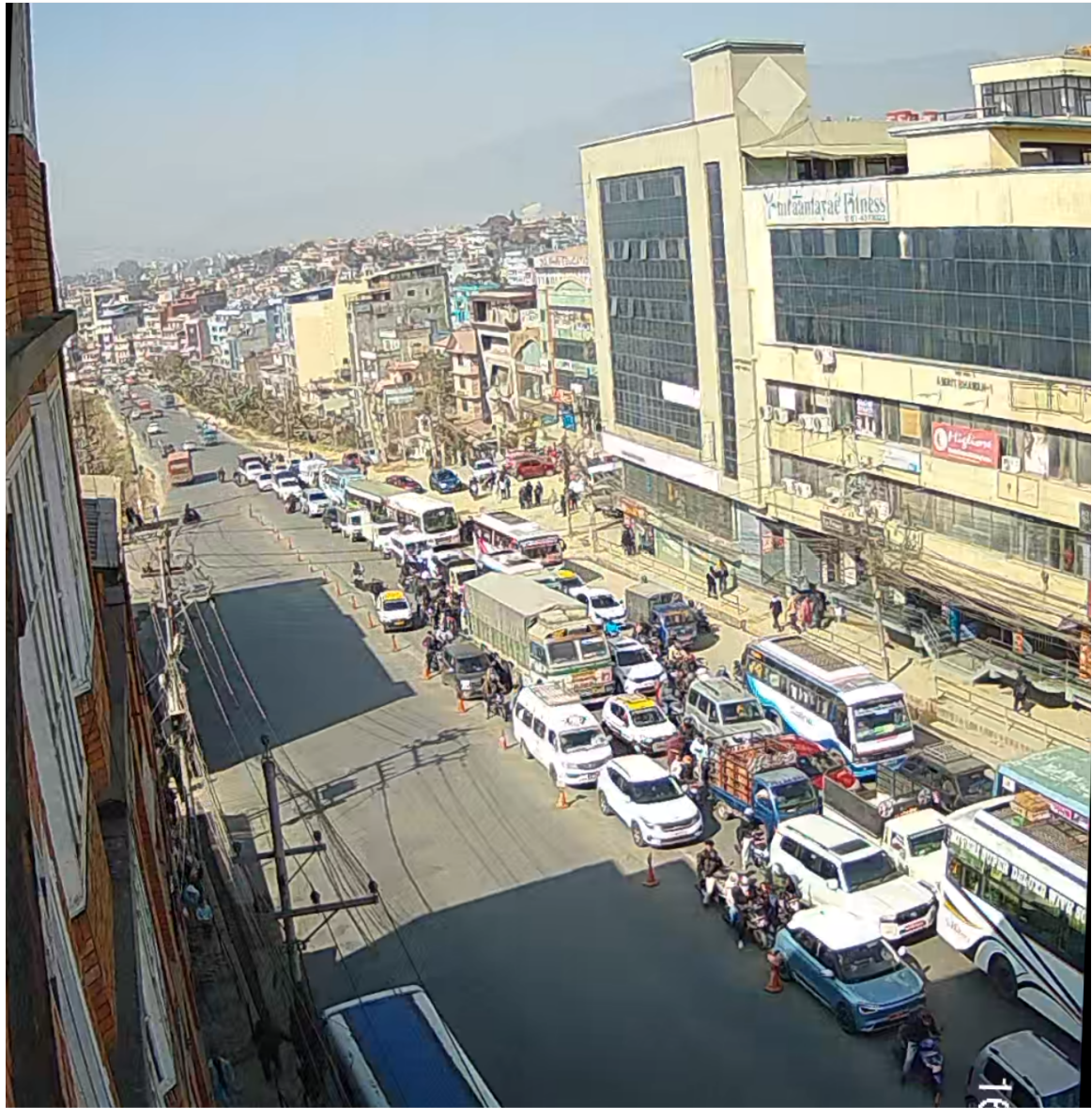
Figure 4.12: Field observed maximum back of queue formation at the Basundhara approach of Narayan Gopal Chowk during the 11-cycle validation window (16 January 2026, 12:15-12:20 PM)
