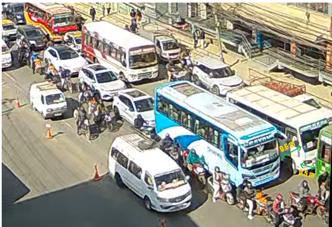
Figure 4.5: Homography-based measurement workflow for extracting heavy-vehicle gaps from CCTV (16 January 2026, 03:00–03:05 PM)
