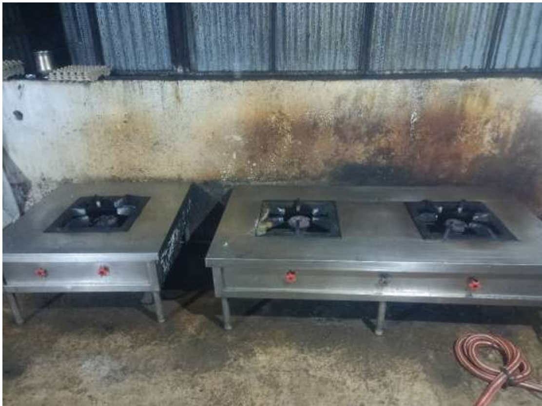
Figure 4.2: LPG burner used for cooking in Sundarijal Arsenal barrack (Burner 1 on the left, Burner 2 on the middle and Burner 3 on the right)
