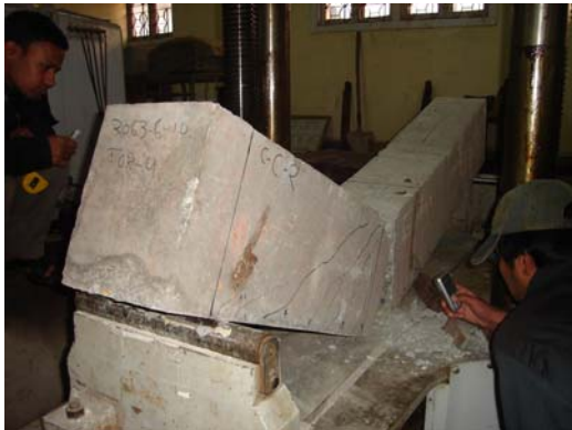
Photo 29: Failure of Beam C-C-2
