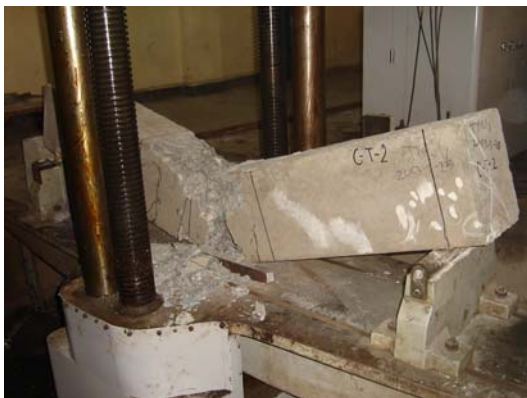
Photo 25: Failure of Beam C-T-2
