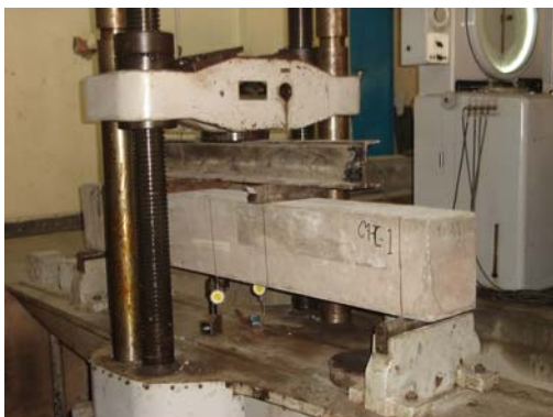
Photo 13: Beam Setup on UTM
