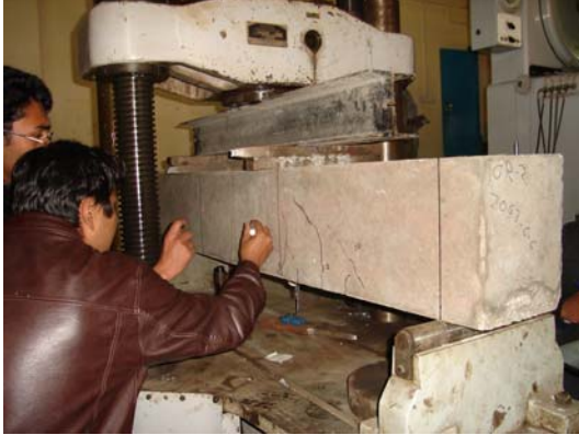
Photo 21: Marking Crack in Beam M-C-2
