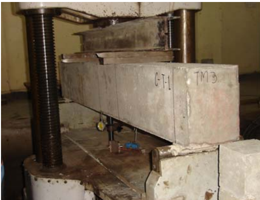
Photo 23: Setting Beam C-T-1 on UTM table
