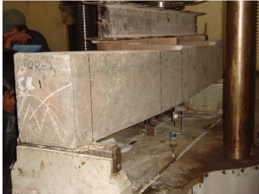
Photo 27: Loading on Beam C-C-1
