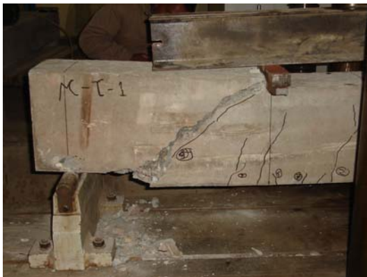
Photo 19: Shear Failure of Beam M-C-1
