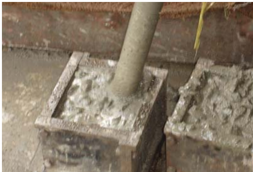
Photo 11: Concreting Cube with vibration
