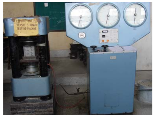
Photo 14: Compressive Strength test of Cube
