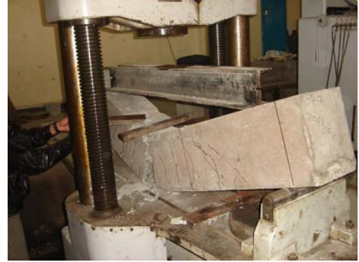
Photo 22: Failure of Beam M-C-2
