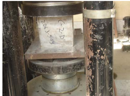
Photo 26: Cube of Beam C-T-2 Testing for Compressive Strength
