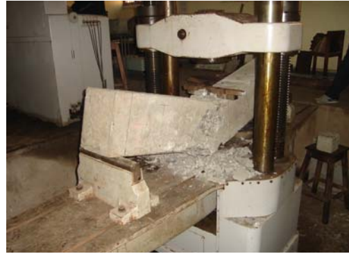
Photo 16: Failure of Beam M-T-1
