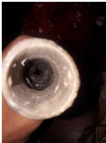
Figure 4.38: Bush nozzle with Mseal as convergent and divergent Section
