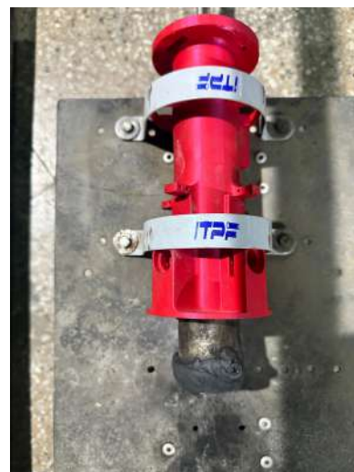
Figure 5.3: Servo housing and composite motor after static thrust test
