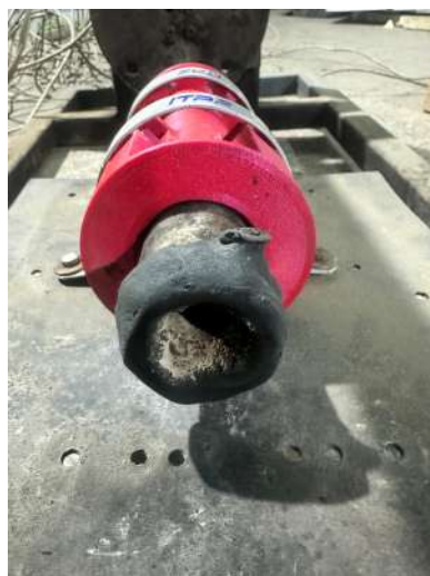
Figure 5.3: Servo housing and composite motor after static thrust test
