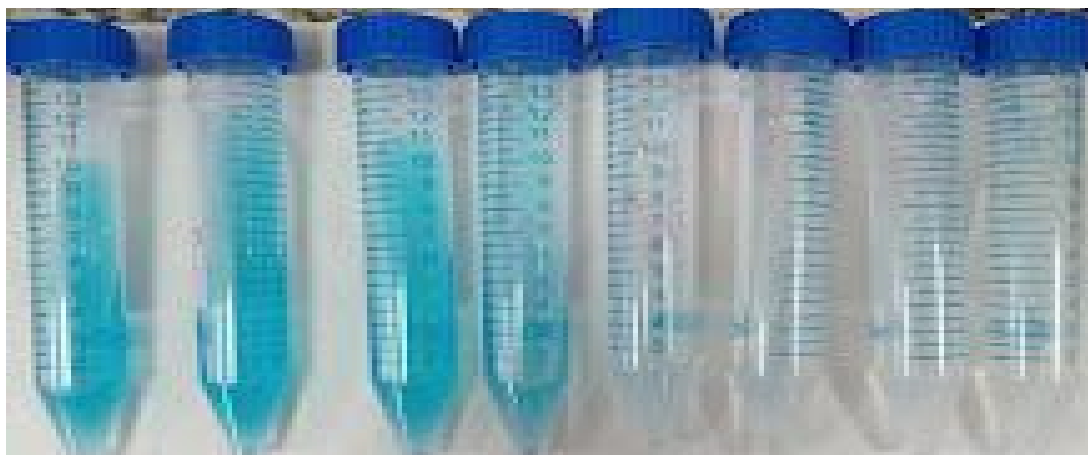
Fig 11 : Visual Observation of gradual degradation of MB in CoCe(3)-ZnO For methylene blue (MB), the characteristic peak is around 664 nm. The absorbance values obtained from UV-Vis spectroscopy for each of the samples are tabulated in Table 4
