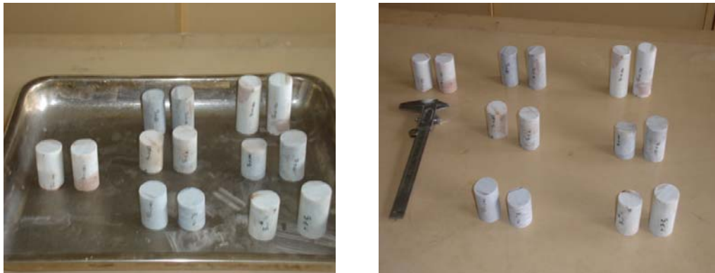
Fig. 5.9 Core samples for the determination of dry density and water absorption.
