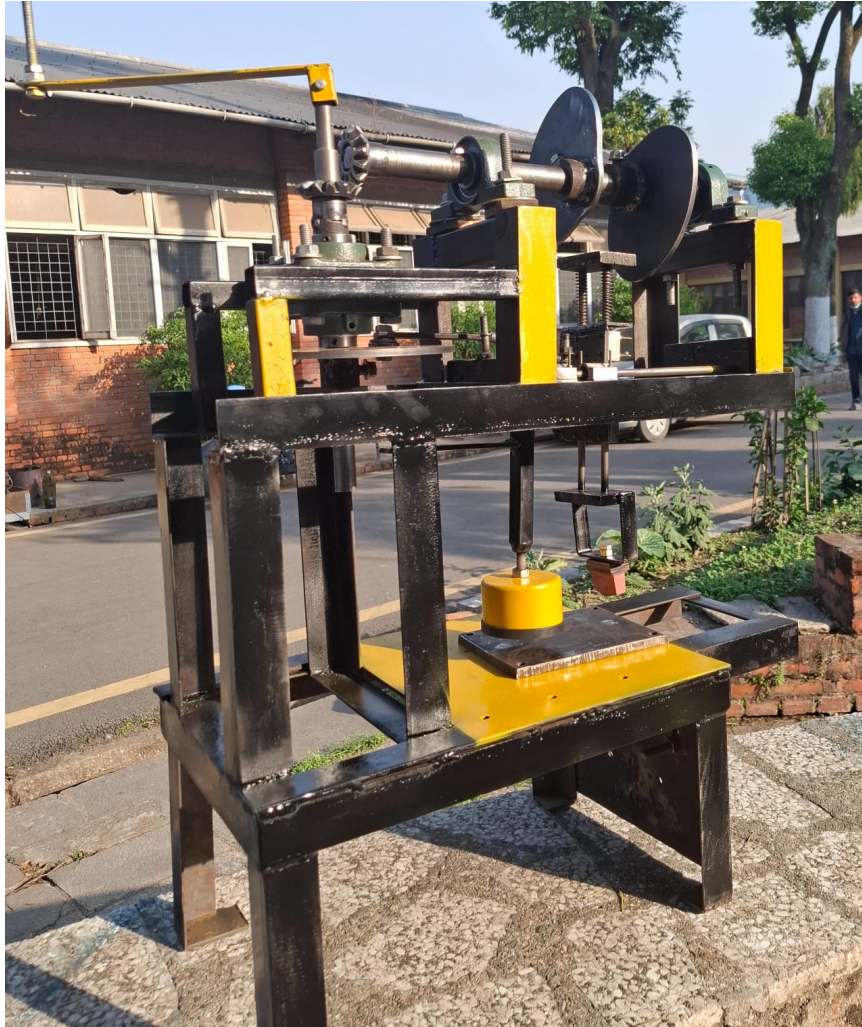
Figure 4.15: Pad Printing Machine
