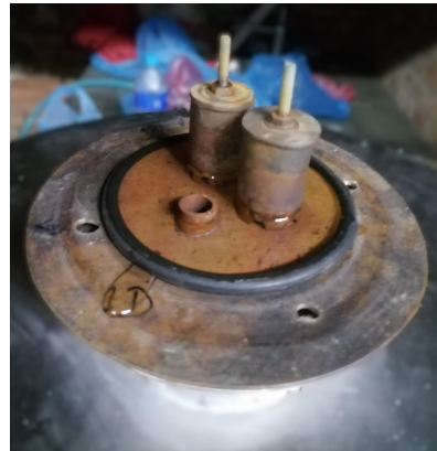
Fig. A15: Bubble Cap Tray after use
