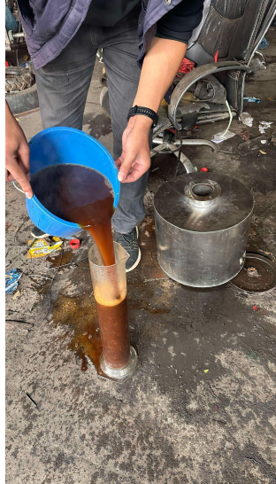
Fig. A16: Volumetric Measurement of remaining Fermented Mass
