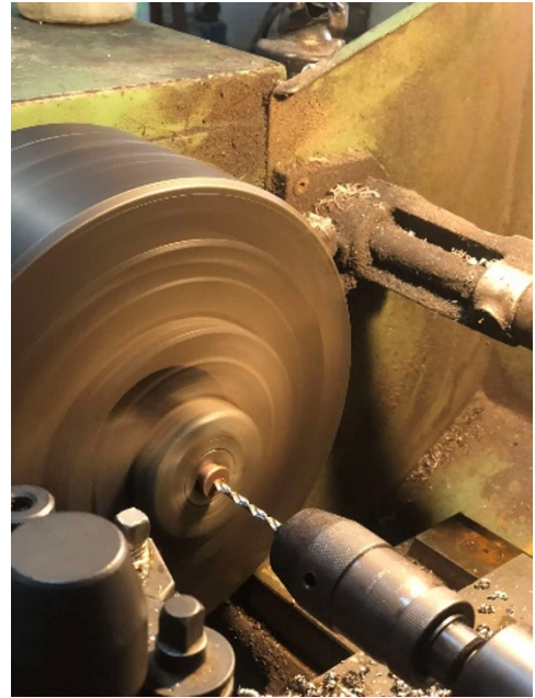
Fig. A13: Drilling of Bubble Caps
