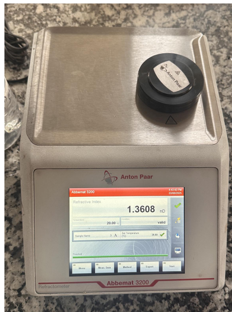
Fig. A19: Testing Alcohol Concentration using Refractometer
