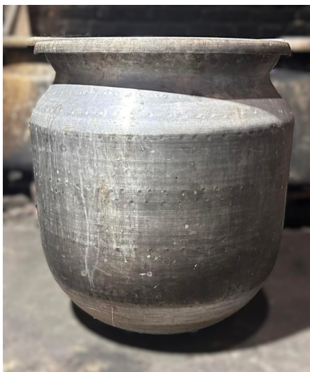
Fig. A3: Paini (Condensation Chamber)
