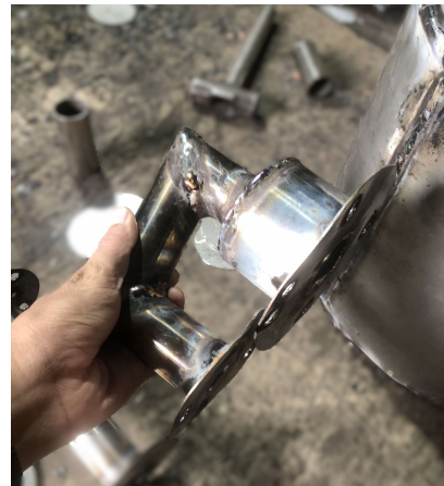
Fig. A11: Reflux Condenser manufacturing
