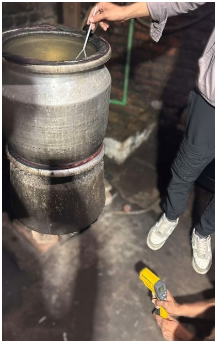
Fig. A6: Measurement of condensing water temperature
