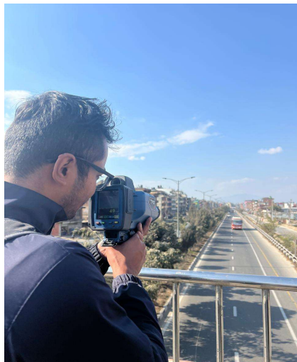
Figure 3.8: Speed data collection using LiDAR
