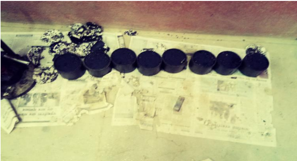
Photograph 0-8 Marshall Sample of New Graded Aggregate with Varying RAP
