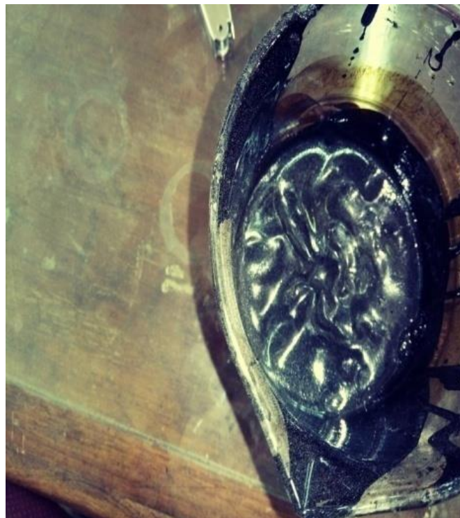
Photograph 0-3 Extraction of Bitumen from RAP
