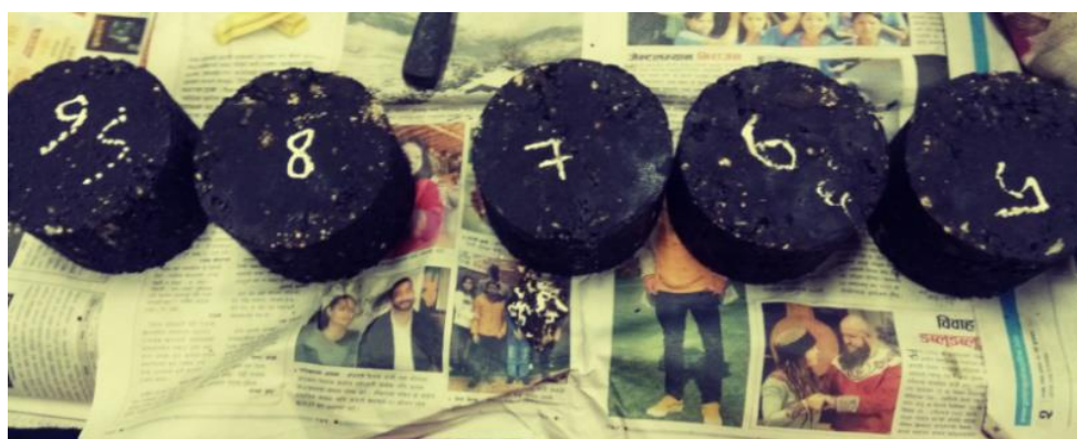
Photograph 0-7 Marshall Sample Preparation and Testing of Virgin Mix
