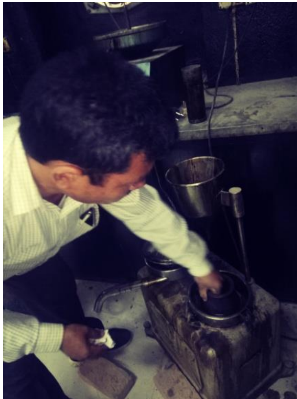
Photograph 0-4 Extraction of Aggregate from RAP Sample
