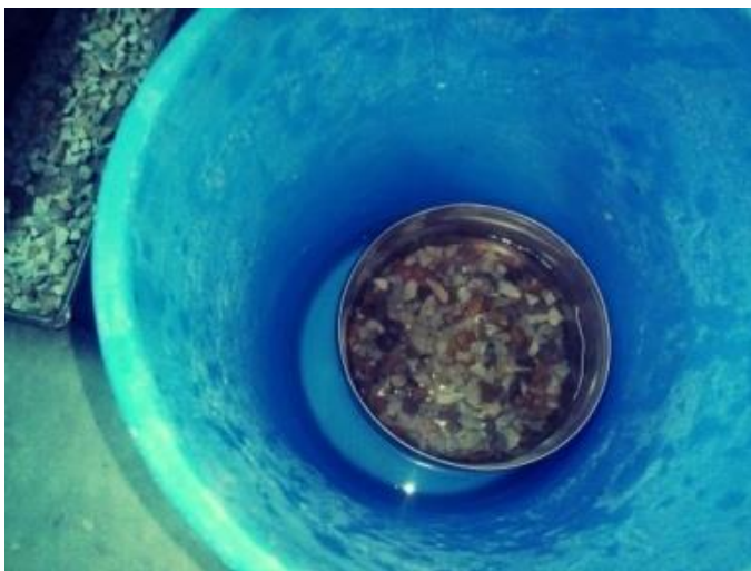
Photograph 0-5 Sodium Sulphate Soundness and Striping Test of New Aggregate
