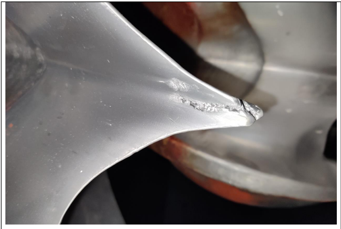
Figure 3.4: On long run, tip erosion due to cavitation
