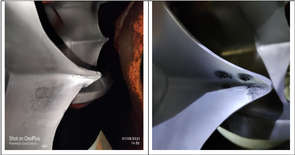
Figure 3.3: After few years run minor effect of cavitation
