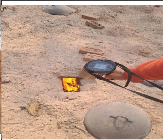
Temperature measurement inside the firing zone
