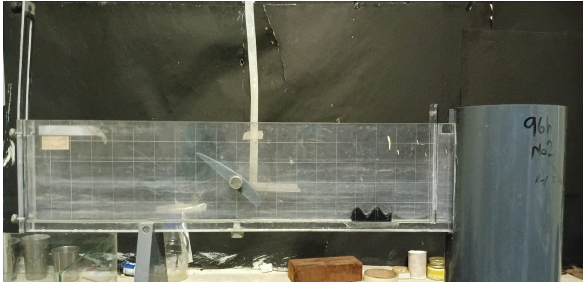
Figure 3.23: Flow Channel with Sinusoidal waveform Structure
