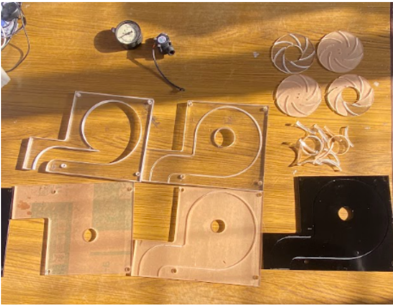
((a)) Fabricated acrylic parts (before assembly)
