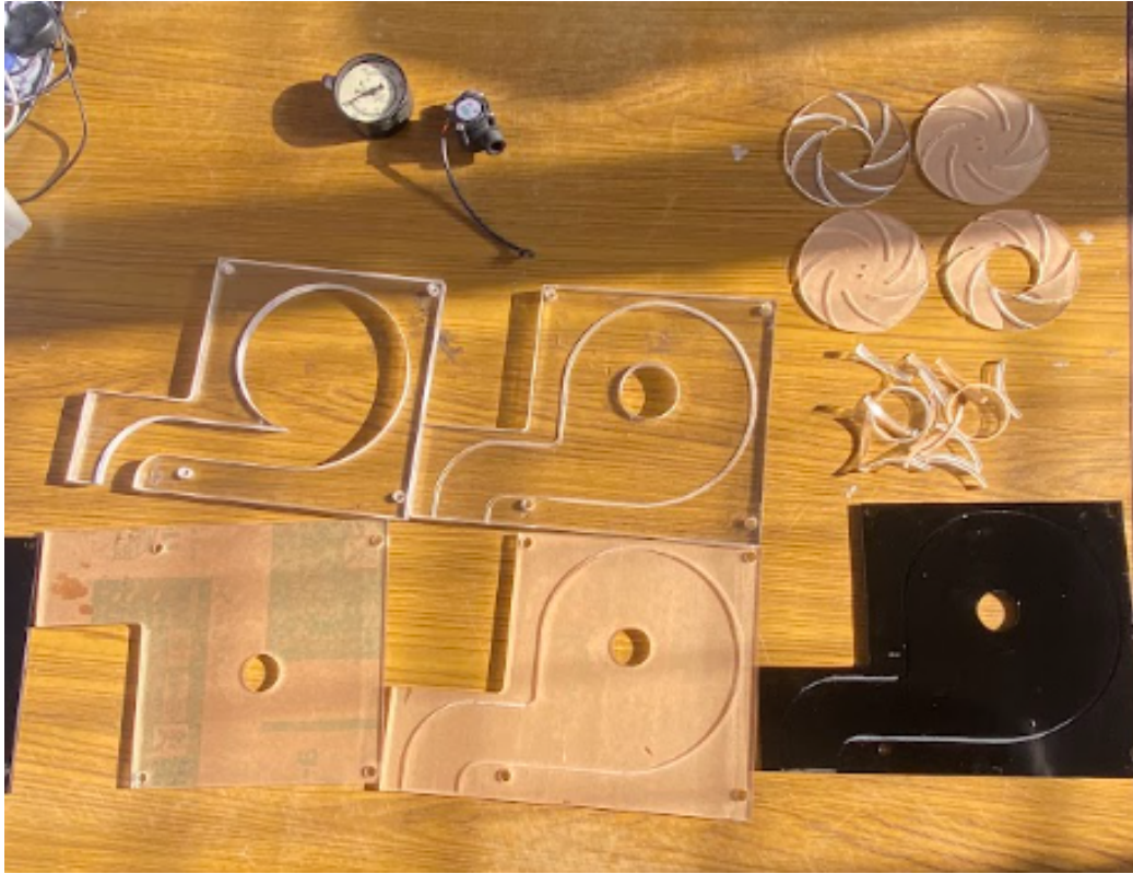
Figure 3.8: Fabricated Acrylic Parts(Before Assembling)
