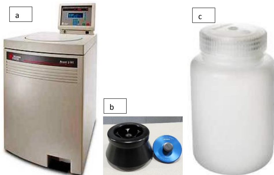
Figures 4.1: (a) Beckman coulter centrifuge (b) JLA-16.250 rotor and (c) Nalgene bottles (500ml) use for centrifugation: these instruments are used to purify desired protein from culture.
