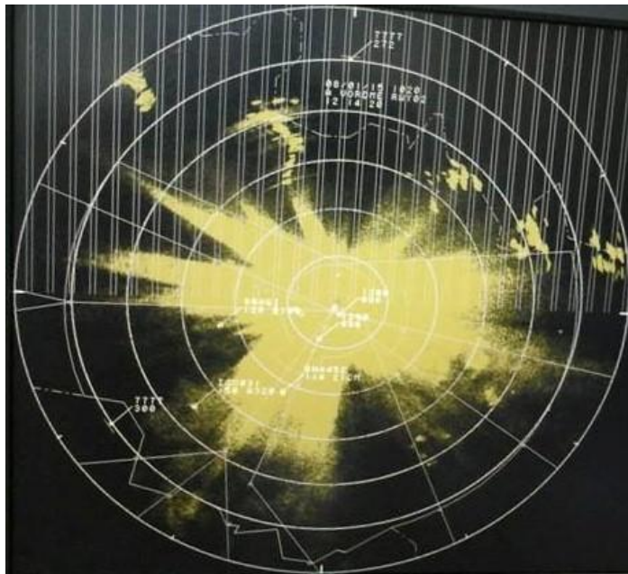
Figure 3.6 PPI screen of an ATC-radar with targets and clutter (Courtesy: Radar Surveillance Division, TIA, Kathmandu, Nepal)
