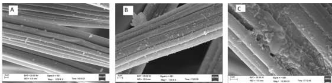
Figure 7: SEM images of graphite electrode. A: Normal graphite electrode, B: Acidified CNT treated graphite electrode and C: Acidified CNT treated graphite electrode after MFC operation.
