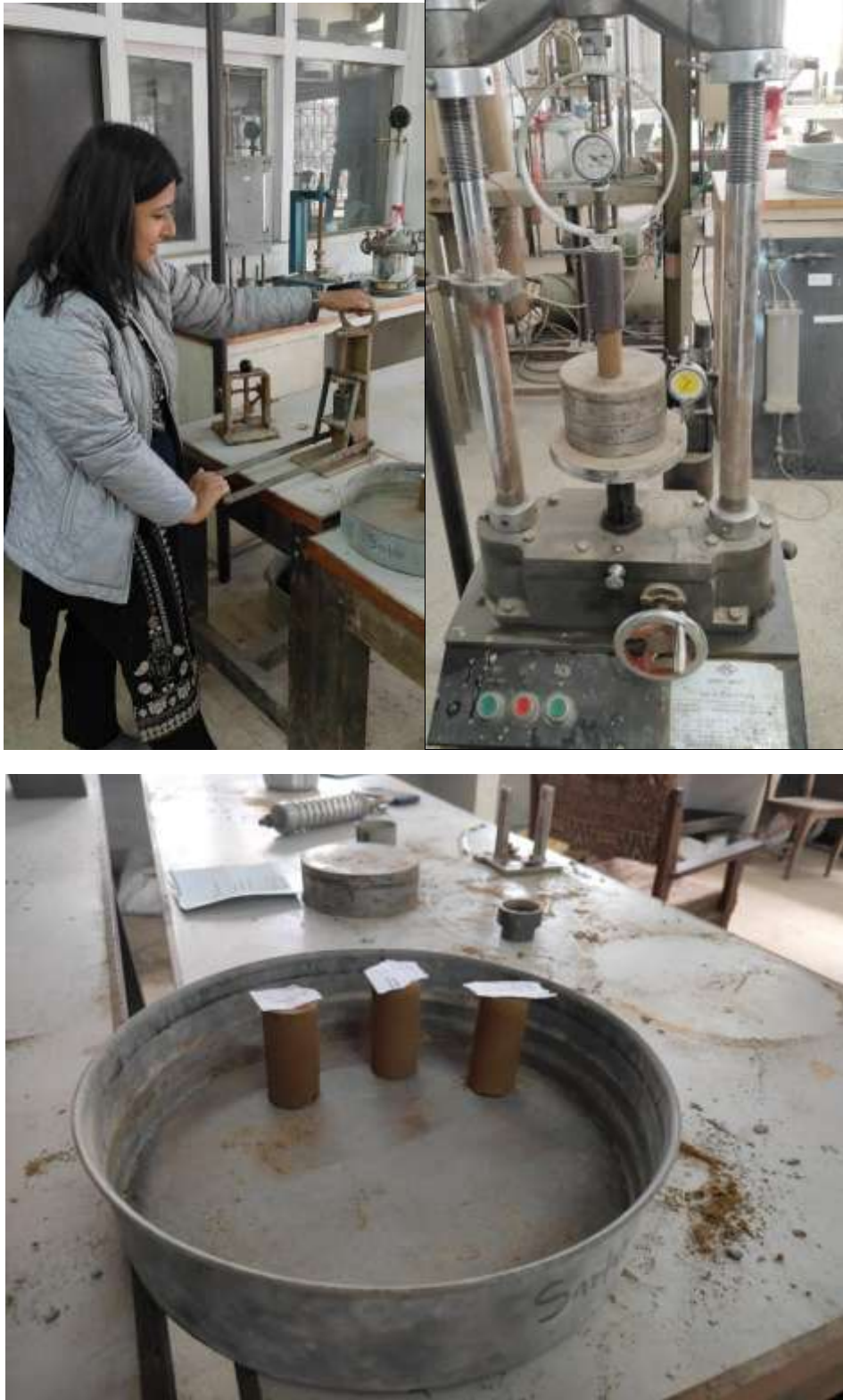
Figure F5 Unconfined Compression Test of Remolded Soil Samples Taken from 1+700CH and 1+800CH: Sample Extraction (Left Figure); Test Setup (Right Figure); Remolded Soil Samples (Bottom Middle Figure)
