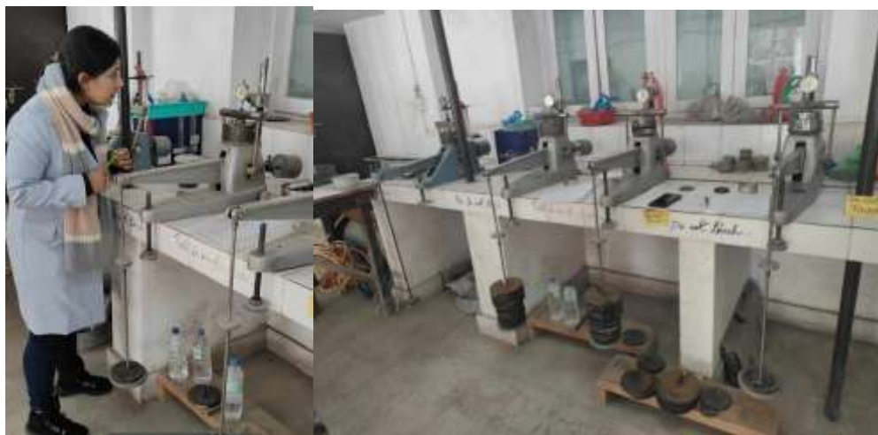
Figure F4 Consolidation Test of Soil Samples Taken from 1+700CH and 1+800CH: Overall Setup (Left Figure); Placement of Soil Samples from 1+700CH and 1+800CH (Right Figure)
