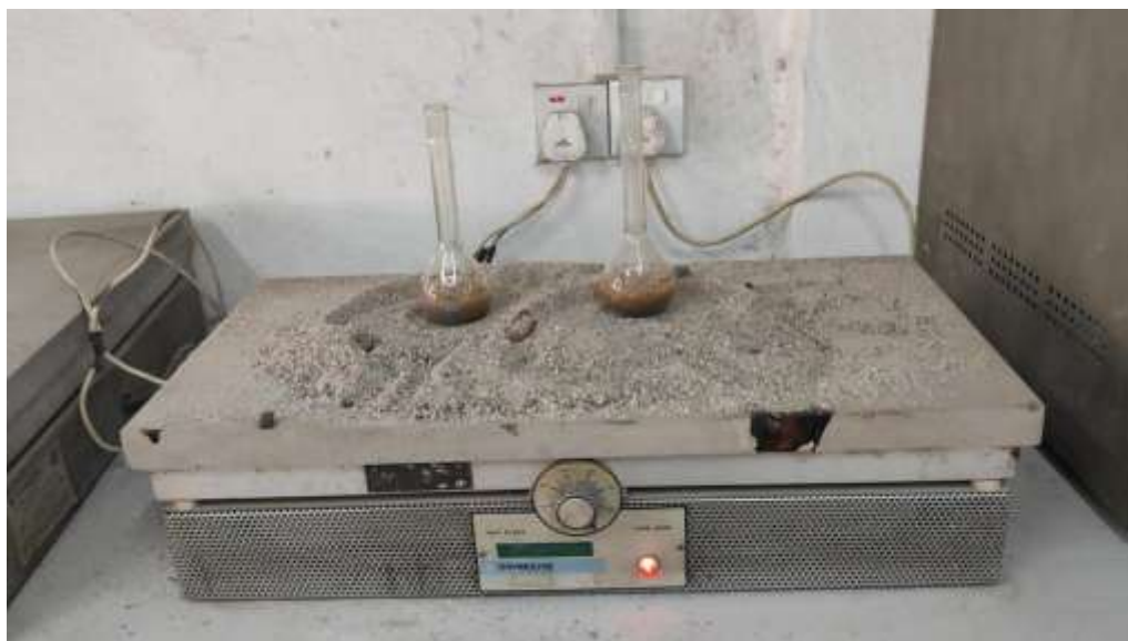
Figure F9 Specific Gravity Test: Sample Preparation (Left Figure); Dry in Sand Bath (Right Figure)
