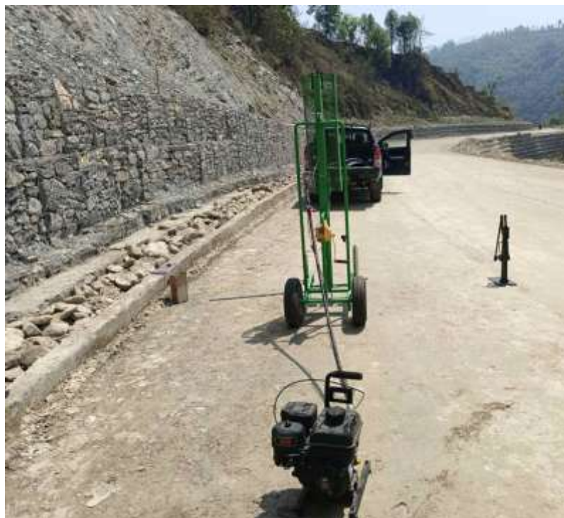
Figure 3.5 Standard Motorized DCPT Dynamic Cone Penetrometer
