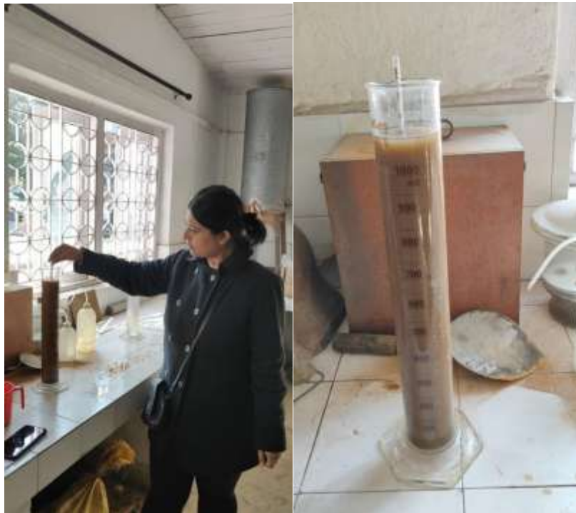
Figure F7 Hydrometer Test: Measurement taken (Left Figure); Sample Preparation (Right Figure)
