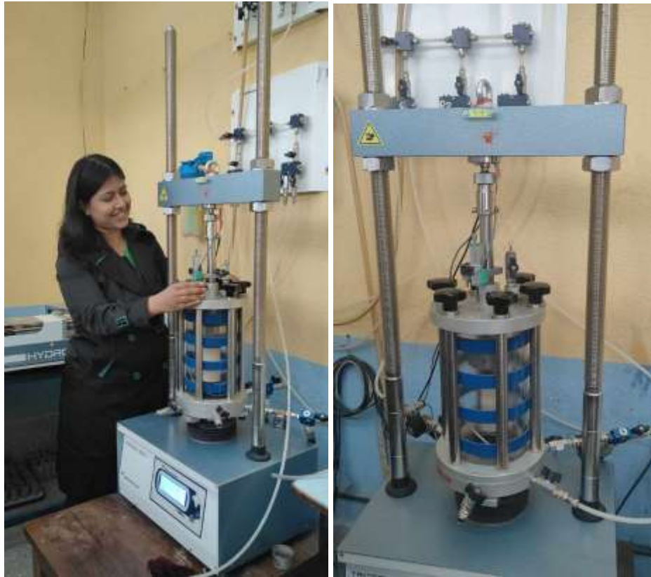
Figure F3 Triaxial Test of Soil Samples Taken from 1+700CH and 1+800CH: Overall Setup (Left Figure); Placement of Soil Sample from 1+700CH (Right Figure)
