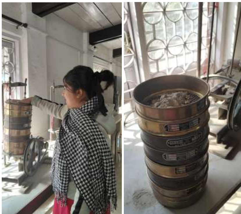
Figure F8 Sieve Analysis: Mechanical shaking (Left Figure); Sample Preparation (Right Figure)
