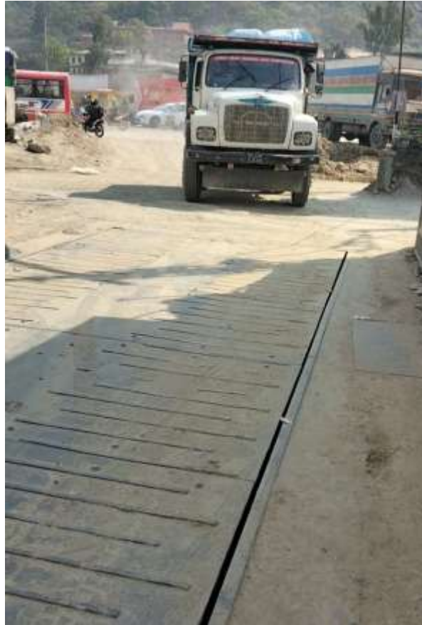
Figure I1. Weighing TATA TRUCK 1613c (Empty Weight: 7745KG)
