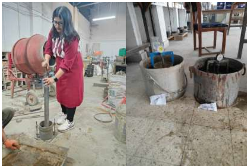
Figure F2 CBR Sample Preparation: Sample Preparation in CBR Mould (Left Figure); Placement of Sample for 72 Hours of Saturation Prior to Testing (Right Figure)
