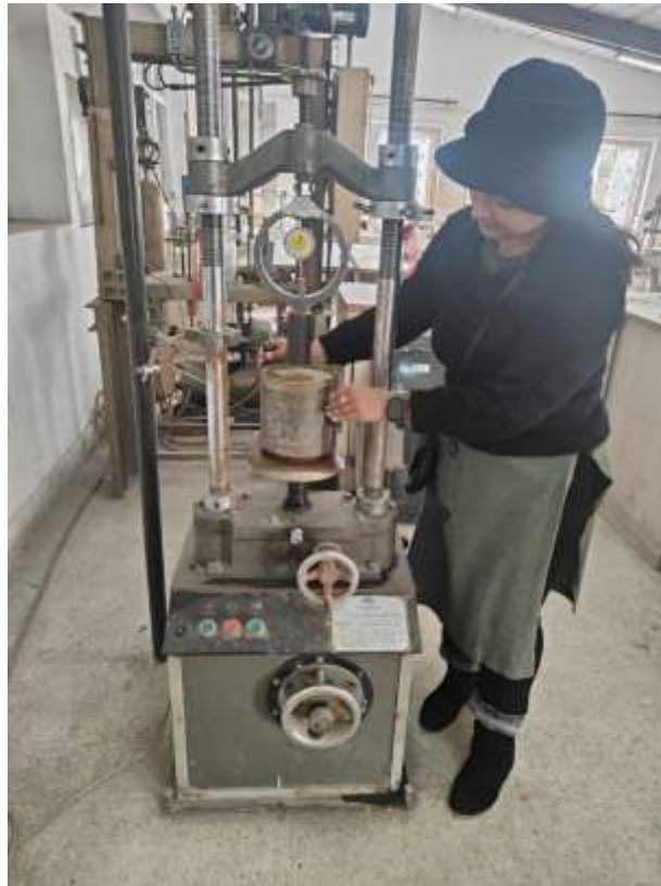
Figure F1 CBR Sample Test Setup for Soil Samples Collected from 1+700CH and 1+800CH
