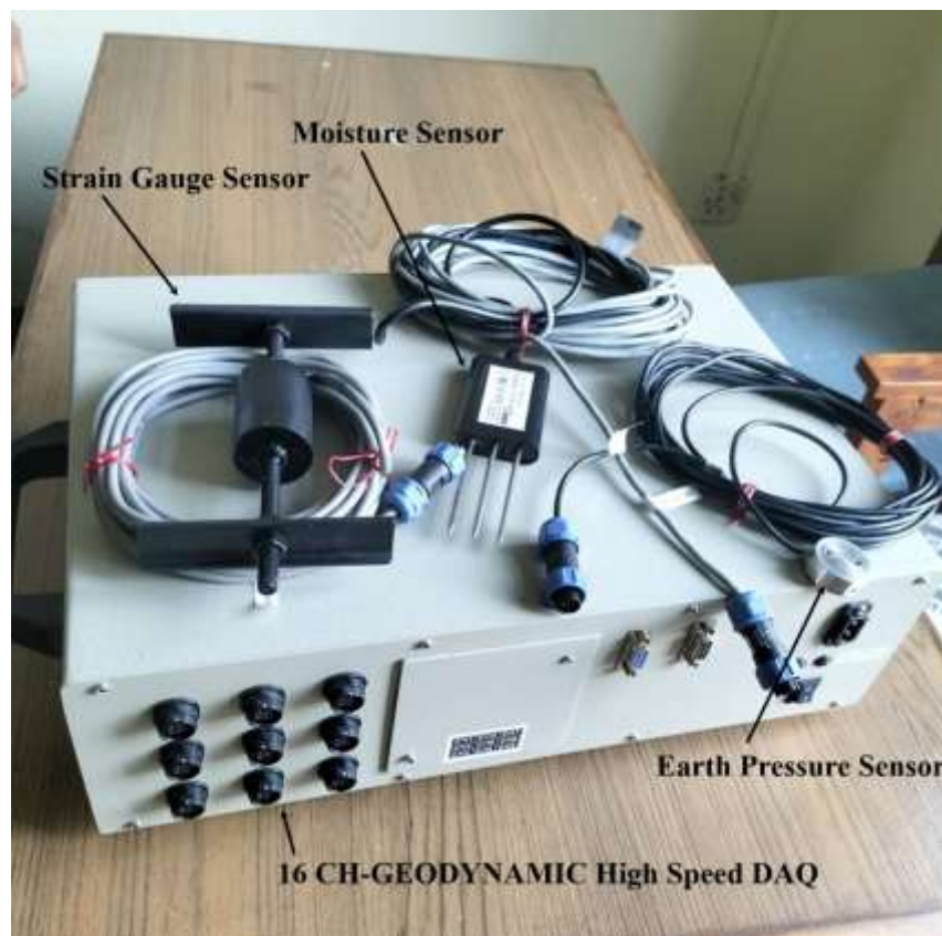
Figure 3.4 Geodynamic High-Speed DAQ with Dynamic Amplifier and Sensors
