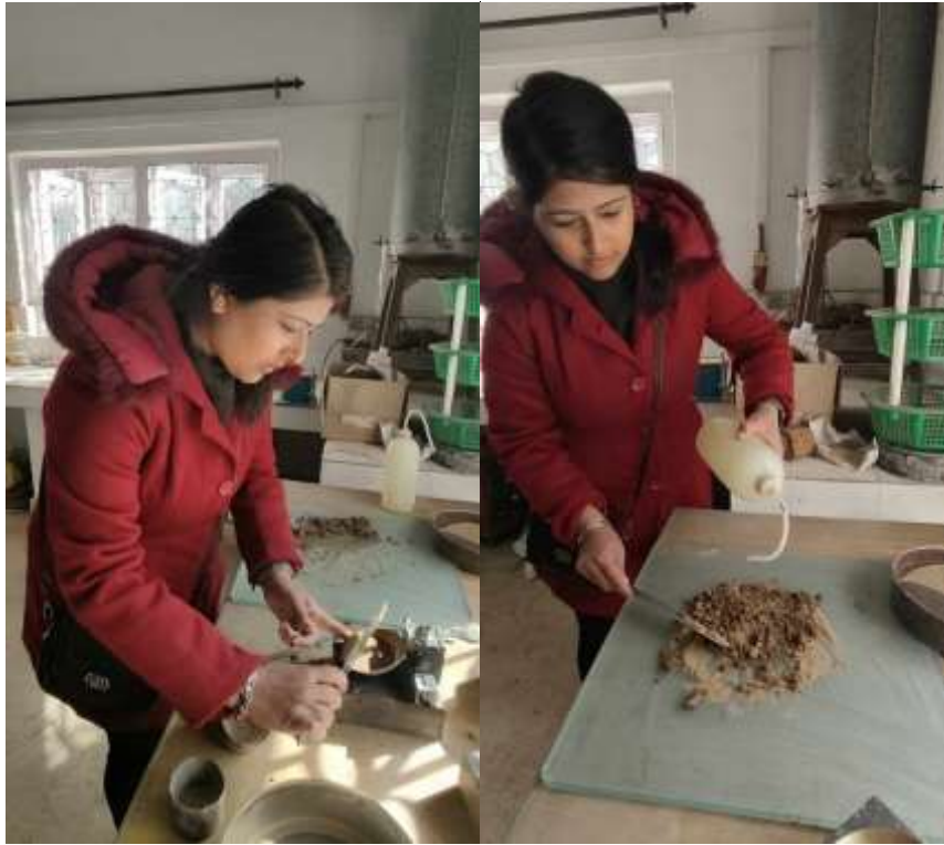
Figure F10 Casagrande Tests for LL and PL Tests: LL test (Left Figure); Soil sample preparation (Right Figure)
