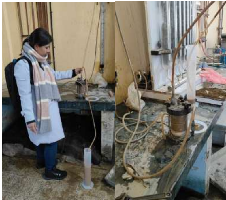
Figure F11 Constant Head Permeability Test: Taking test results Left Figure); Overall Test Setup (Right Figure)
