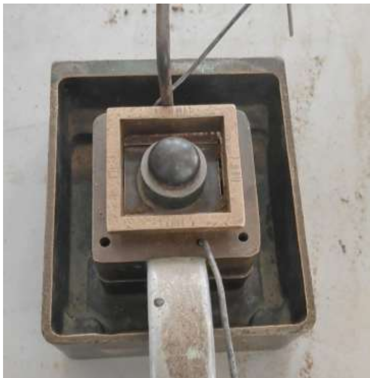
Figure F6 Direct Shear Tests of Soil Samples Taken from 1+700CH and 1+800CH: Overall Test Setup (Left Figure); Sample Preparation (Right Figure)
