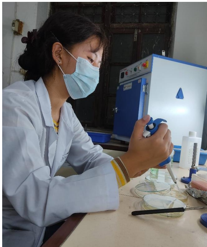
Photograph 4: Inoculation of hand sanitizers using agar well diffusion method
