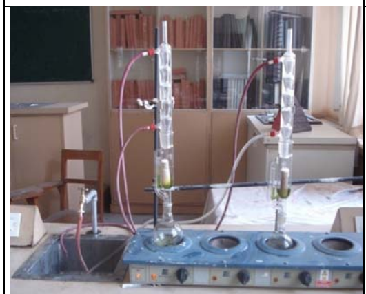
Soxhlet apparatus for extraction of phenol and essential oil
