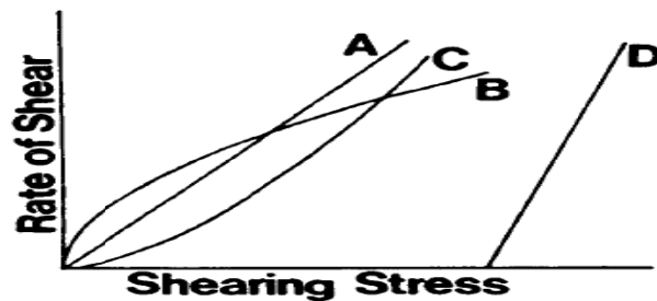
Fig.3.27. Shearing stress-rate of Shear digram, (A) Newtonian, viscous flow, (B) Dilatant flow (C) Pseudoplastic flow, (D) Plastic flow.
