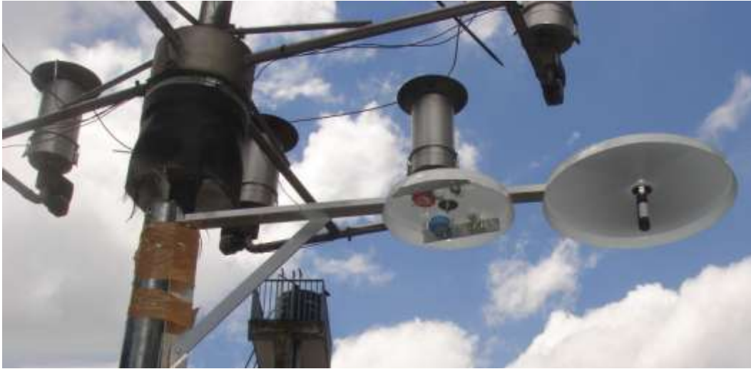
Figure 4.4: Exposure of Passive samplers mounting with metal disc as rain shield at Thamel.
