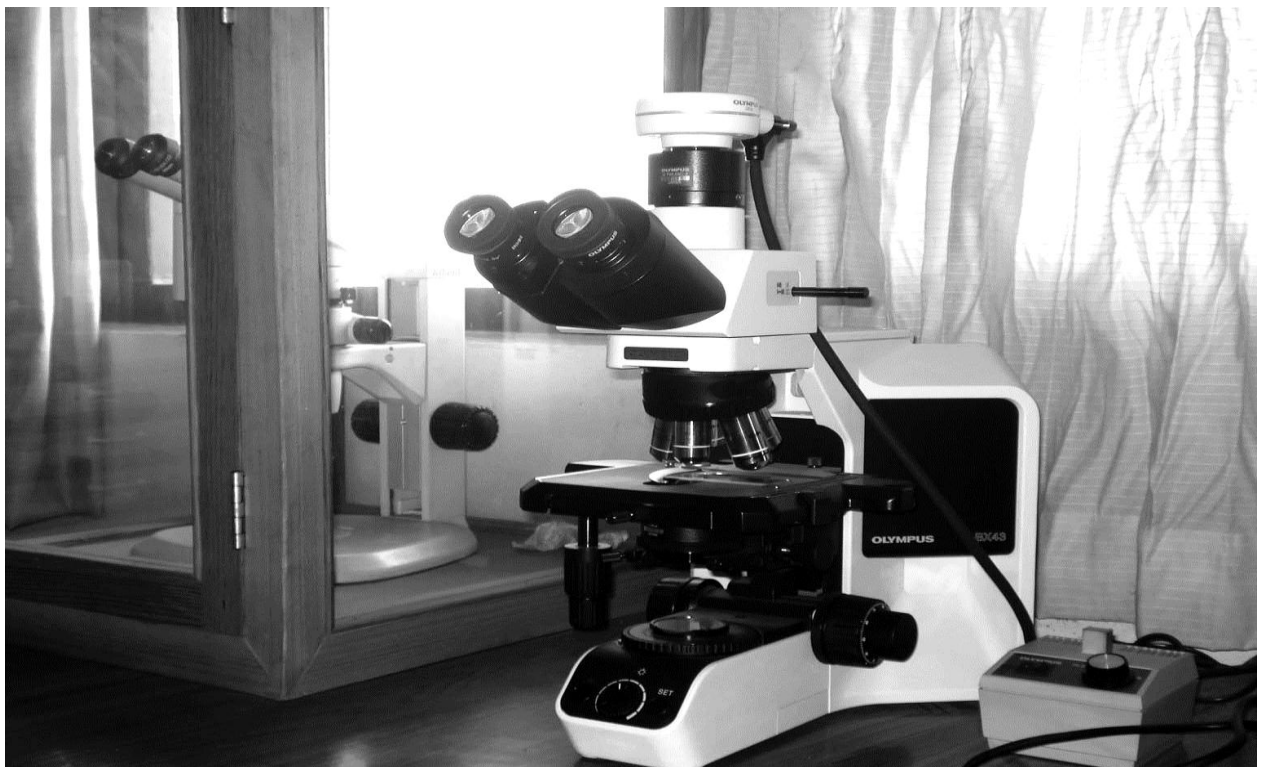
Figure 3: Olympus BX43 microscope for light microscopy for pollen study.
