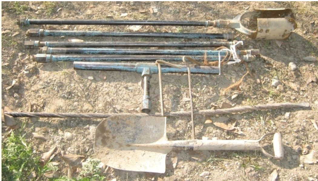
Fig. 3.2: Instruments used in Augering
