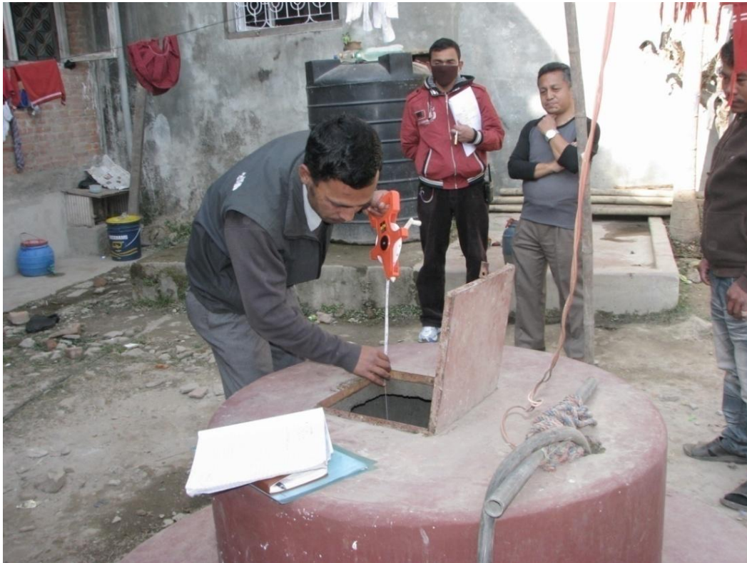
Fig. 3.5: Water Level Monitoring in Wells at United Academy, Kumaripati
