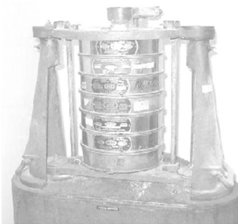
Fig.3.7: A Complete Instrument of Sieve Analysis
