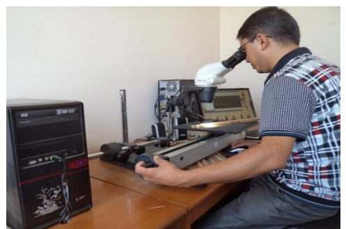
Measurement of ringwidth in the LINTAB system in Dendrolab
