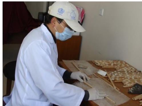
Sanding and polishing of tree core samples
