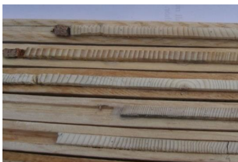
Tree-rings in samples after sanding and polishing
